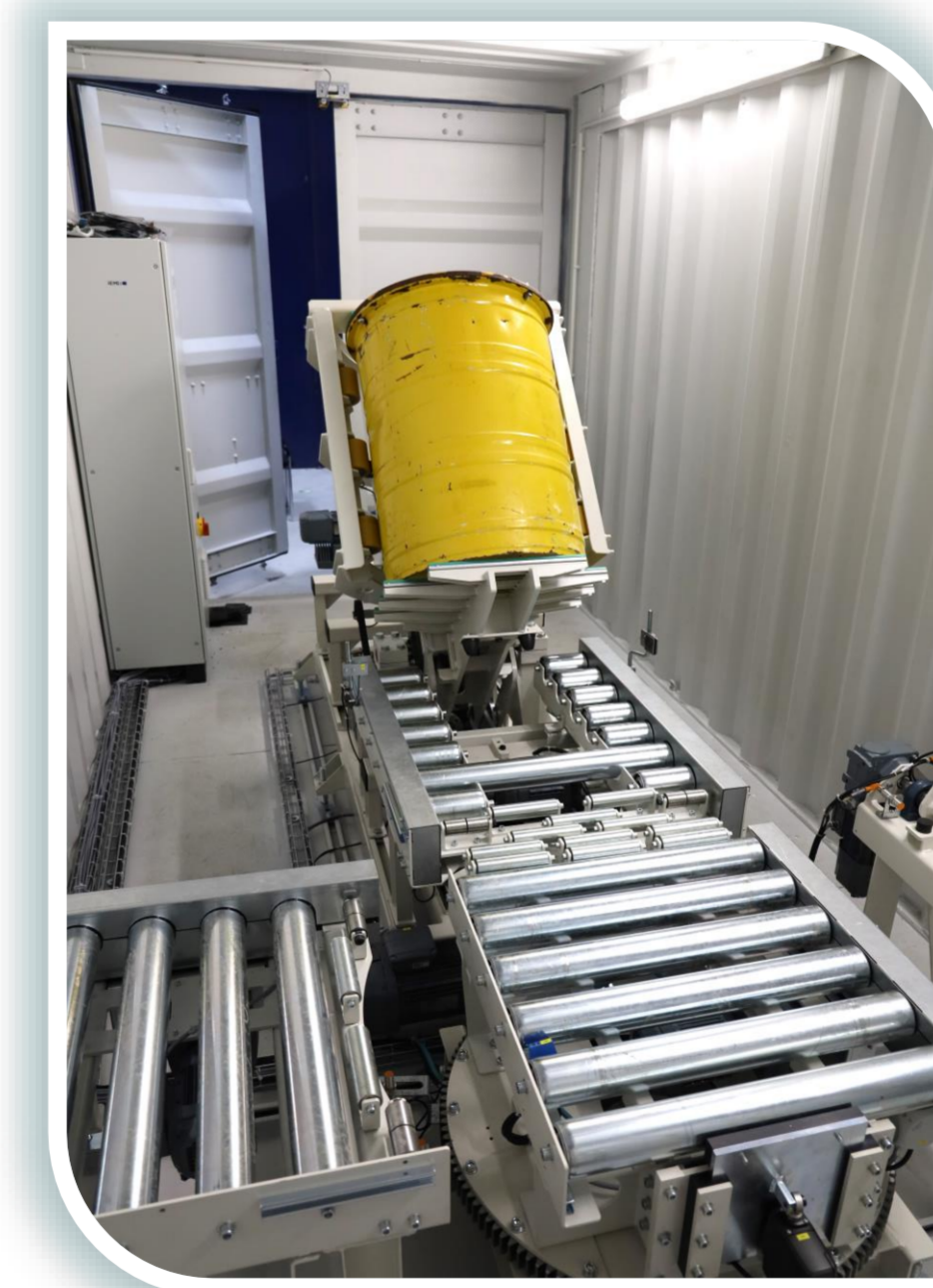
Drum on tipping system
