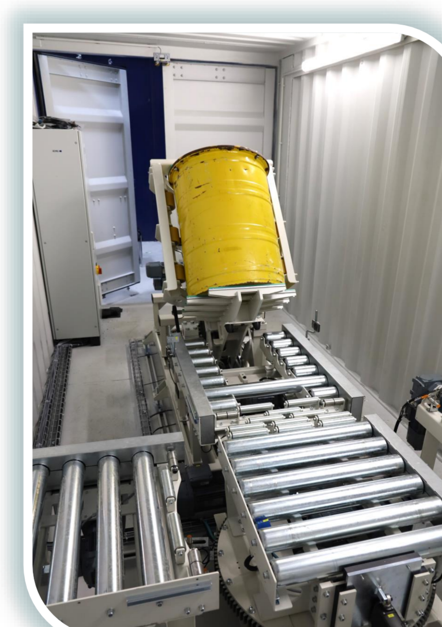
Drum on tipping system
