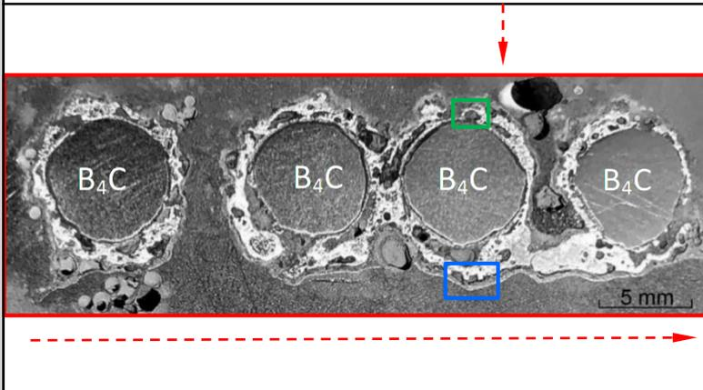
cross section of four B<sub>4</sub>C pins interacted with steel blade
