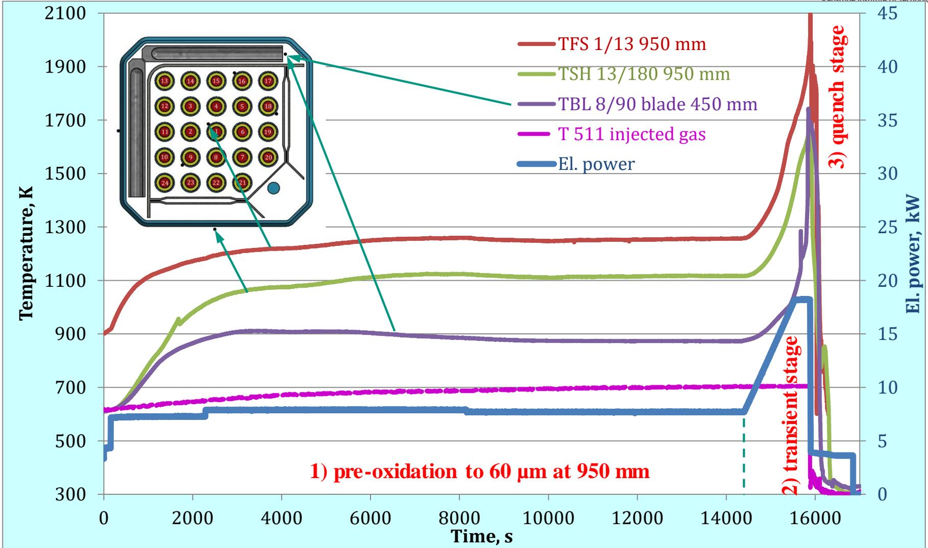
**gas injection: Ar 3g/s during the whole test; superheated steam 3 g/s until the quench initiation**
