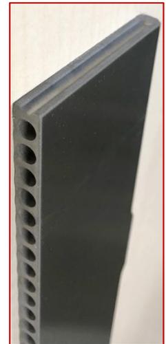
horizontal holes for B<sub>4</sub>C pins
