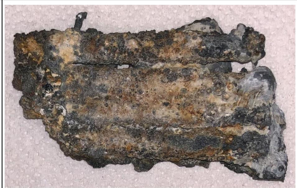
back side view: absorber blade covered by oxidized channel box
