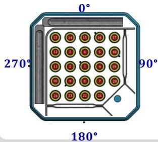
Strong degradation of absorber blades, channel box and shroud between elevations 650 and 950 mm at angle positions 0° and 270°
