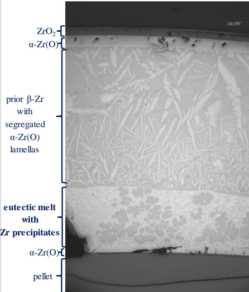
optical observation of cladding at 450 mm
