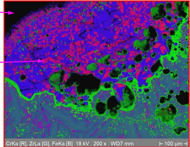
contact B<sub>4</sub>C with steel blade
