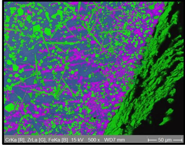
ZrB<sub>2</sub> needle precipitates in Zr-steel eutectic melt
