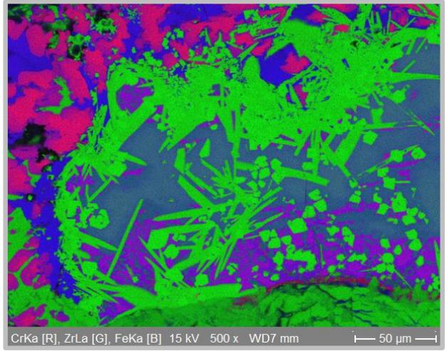
ZrB<sub>2</sub> needle precipitates in Zr-steel eutectic melt
