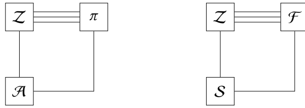
Figure 2.1.: The UC experiment with real adversary \mathcal{A} and protocol \pi (left) and with simulator \mathcal{S} and ideal functionality \mathcal{F} (right). The multiple lines indicate that \mathcal{Z} may interact with multiple protocol parties.
