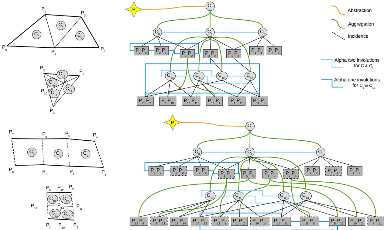
Figure 6. Example of a *Triangle3DComponent* object (top) and *Segment4DComponent* object *C* (bottom) using *Property Graph Model* together with a selection of *G-Maps* involutions (blue).
