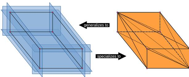
Figure 7. abstraction relation; BLUE: topologically inconsistent *Triangle3DNet* object made off six *Triangle3DComponent* objects; BLACK: surface intersections (left) triangle borders (right); ORANGE: *Tetrahedron3DComponent* object as result of the tetrahedralization
