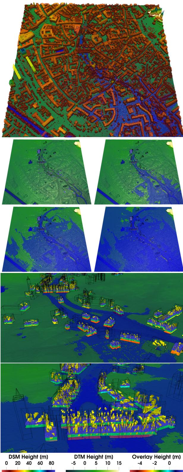
Figure 8. Digital Surface Model (DSM, coloured by height), Digital Terrain Model (DTM, coloured by height), CityGML (black), tetrahedralized CityGML (yellow) with shrunk tetrahedra, water surface (blue) at different times and intersection-geometries for each time (coloured by height).
