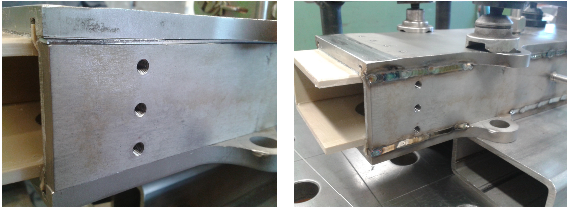
Figure D.1: Photographs of the test section inlet. On the left before welding, on the right after welding. The PEEK inner channel was not compromised during the welding activities per se. However, during the test section transport, one PEEK wall was damaged, as seen in the right photograph.
