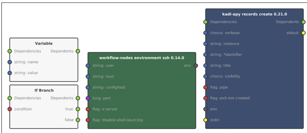
**Figure 6** Available node types. Built-in nodes are grey, environment nodes green and tool nodes blue.
