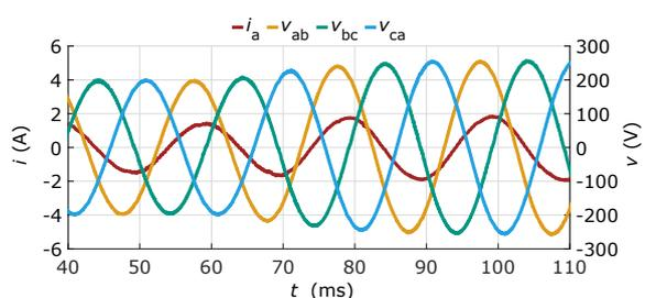
Fig. 12: Measurement of grid forming voltage step
