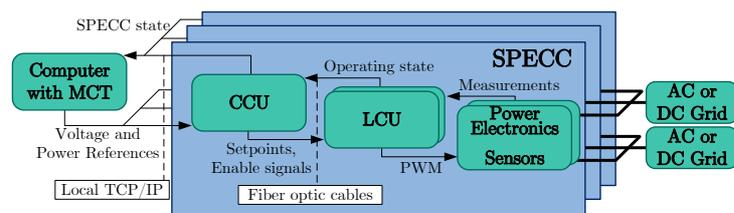
Fig. 3: Hierarchy and interconnections of the signal processing structure
