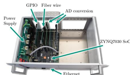
Fig. 4: CCU, based on a ZYNQ7030 SoC
