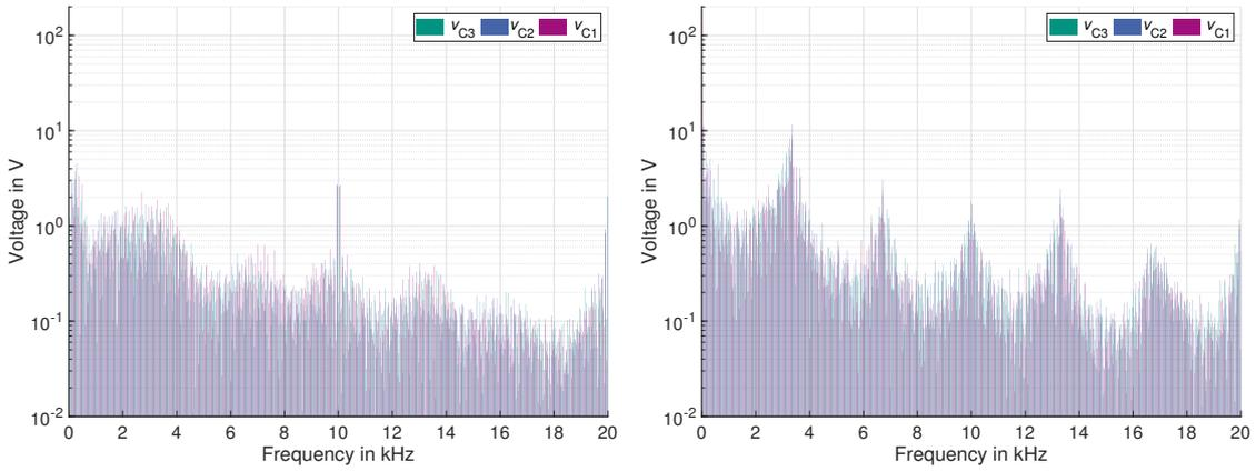
(a) Frequency spectrum of the first methods [5] balancing algorithm - fixed switching sequences and different time  $t_p$  (b) Frequency spectrum of the second methods [4] balancing algorithm - variable switching sequences and fixed time  $t_p$
