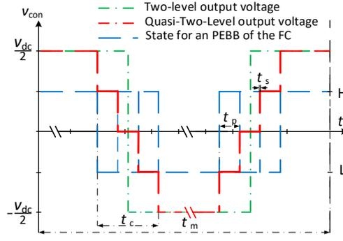
(b) Quasi-Two-Level output voltage principle
