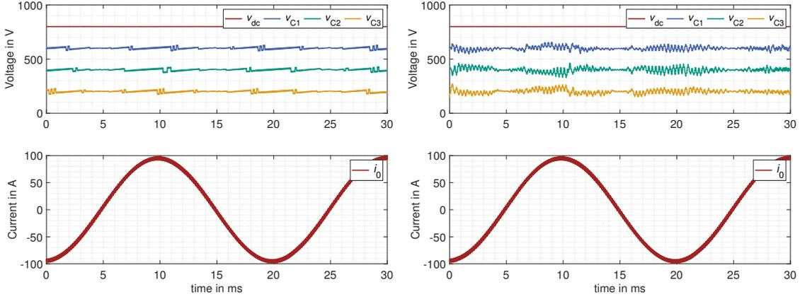
(a) Simulation results of the first methods [5] balancing algorithm - fixed switching sequences and different time  $t_p$  (b) Simulation results of the second methods [4] balancing algorithm - variable switching sequences and fixed time  $t_p$
