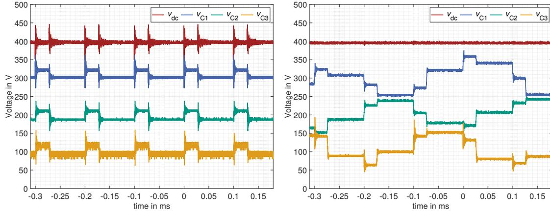
(a) The measured capacitor voltage of the first methods balancing algorithm - fixed switching sequences and different time  $t_p$  (b) The measured capacitor voltage of the second methods balancing algorithm - variable switching sequences and fixed time  $t_p$
