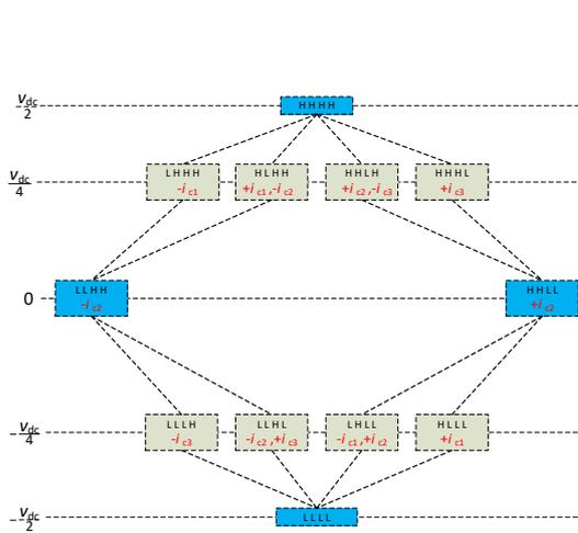
(a) Switching state chart for a 5-level flying capacitor for Quasi-Three-Level Operation
