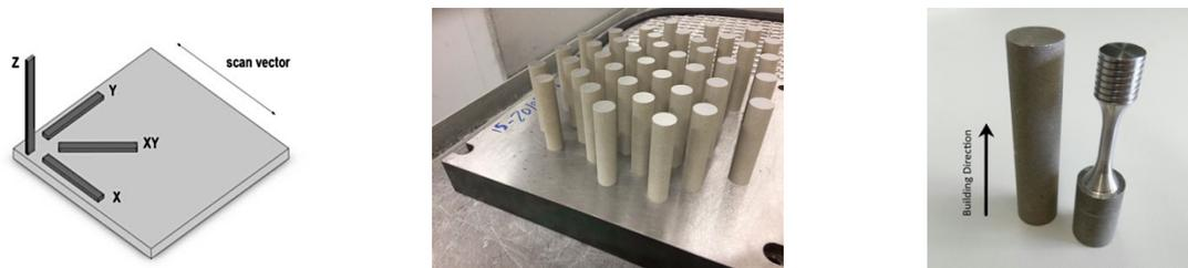
**Figure 2.** Details of specimen printing. Left: printing directions, focus on z-direction; mid: cylinders after printing; right: example of fatigue specimen machined from cylinder.
