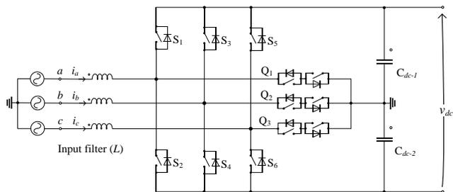
Fig. 9. T-type NPC converter. The fully controlled switches  $Q_1$ ,  $Q_2$ , and  $Q_3$  are implemented with anti-series semiconductors. It is necessary to clamp the neutral point, replacing the clamping diodes of the conventional NPC.
