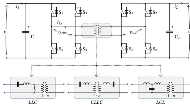
Fig. 12. Resonant cells applied in conventional dual-active bridge converters, including the *LLC* cell, *CLLC*, and *LCL*, highlighted in the power converter circuits.
