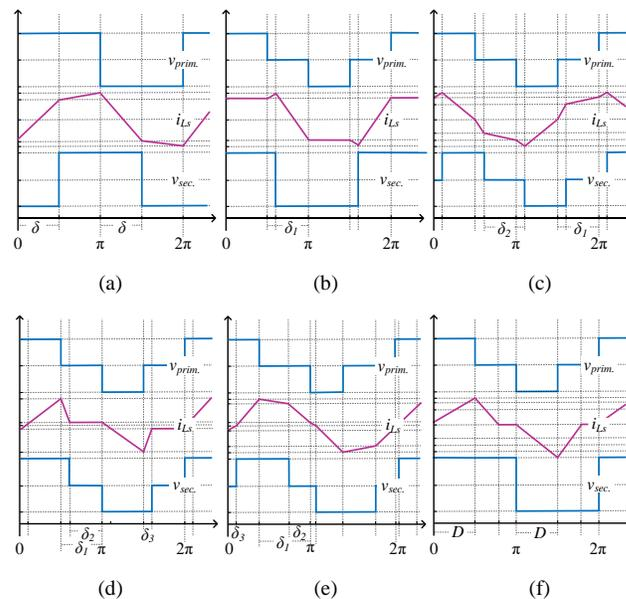
Fig. 11. Non-resonant dual-active bridge converter modulation strategies: (a) phase-shift modulation (PSM); (b) extended phase-shift modulation (EPSM); (c) dual phase-shift (DPSM); (d) triangular triple phase-shift (TRM); (e) trapezoidal triple phase-shift (TZM); (f) pulse-width modulation (PWM). Here the current ( $i_{L_s}$ ) waveforms depend on the phase angles ( $\delta_i$ ) and could be different according to the power processed levels.
