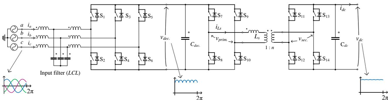
Fig. 15. Power circuit of the two-stage i-AFE converter based on a two-level voltage source converter and non-resonant dual-active bridge (2L-VSC + DAB).
