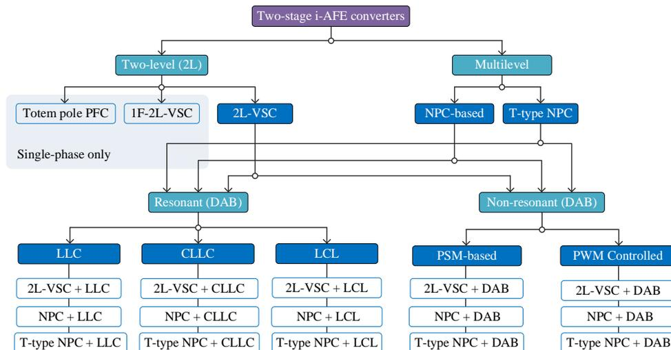
Fig. 14. Classification of two-stage i-AFE converters according to the possible topologies for the PFC stage and isolated dc-dc.
