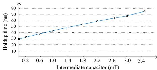
Fig. 27. Evaluation of the holdup time considering different values for the intermediate capacitor according to the results of [121], which considers a 5 kW dc system.
