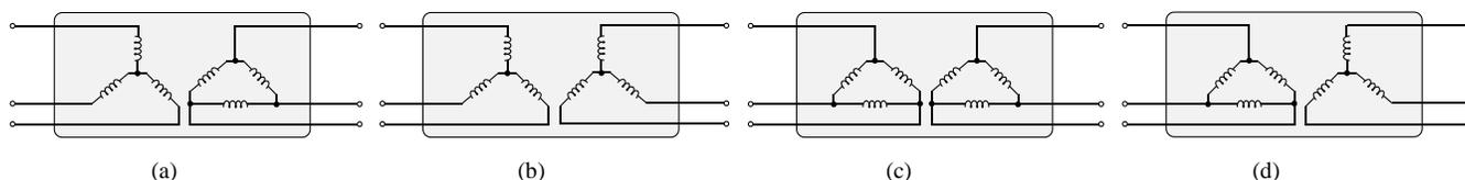
Fig. 17. Possible connections for the high-frequency transformer in the three-phase dual-active bridge converter: (a) Y- $\Delta$ ; (b) Y-Y; (c)  $\Delta$ - $\Delta$ ; (d)  $\Delta$ -Y.
