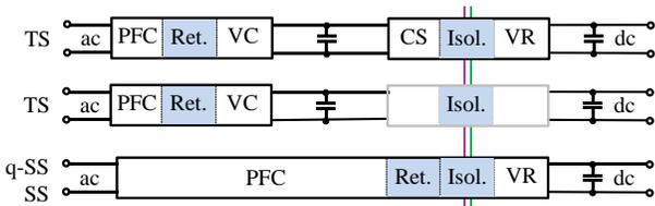
Fig. 25. Distribution of the main tasks required to perform i-AFE conversion, including the power factor correction (PFC), intermediate dc bus voltage control (VC), and voltage regulation (VR) for the output [167].
