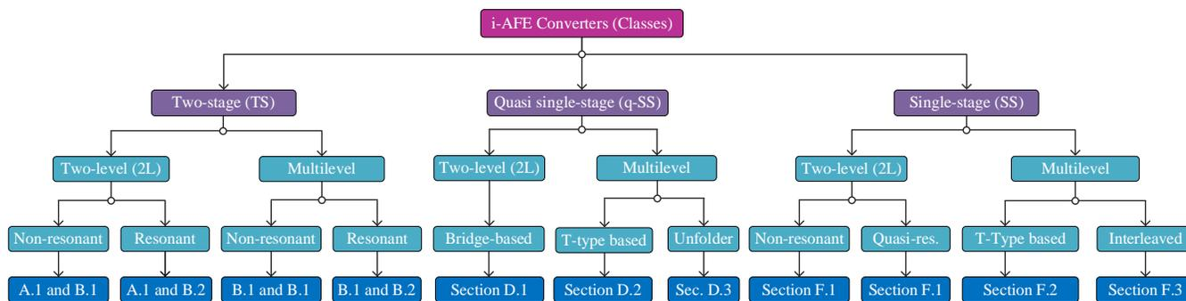
Fig. 6. General classification of i-AFE converters according to the power processing stages and possible topologies for ac and dc sides.
