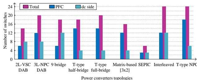
Fig. 26. Comparison of the number of semiconductors for different i-AFE converter topologies.
