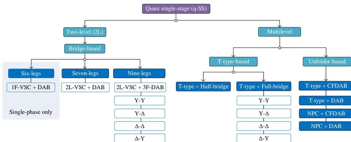
Fig. 19. Classification of the main topologies of quasi-single-stage i-AFE converters.
