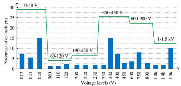
Fig. 3. Common dc bus voltage in existing applications [14].
