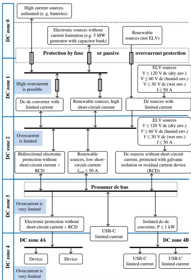
Fig. 4. Safety zones and protection requirements for dc distribution according to NPR 9090 [26].
