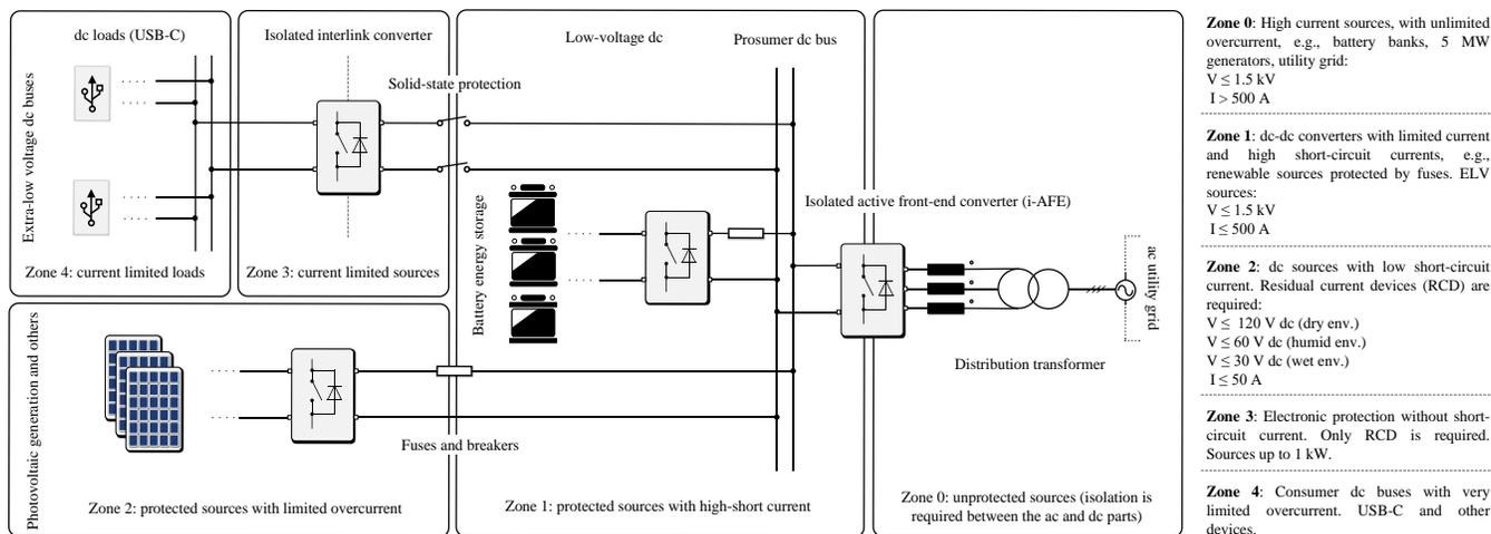
Fig. 1. Interpretation of safety zones in the dc distribution system according to NPR 9090 [1].
