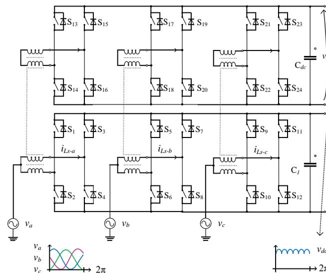
Fig. 22. Power circuit of the three-phase single-stage cascaded full-bridge i-AFE converter.
