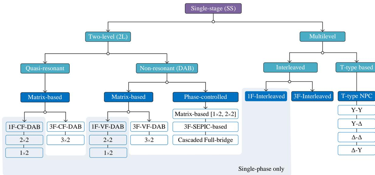
Fig. 24. Classification of the main topologies of the single-stage i-AFE converter.
