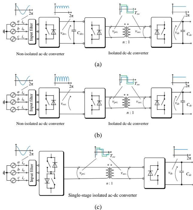
Fig. 2. i-AFE converter solutions: (a) a two-stage (TS) isolated ac-dc converter; (b) no intermediate dc bus required in a quasi-single-stage (q-SS) converter; (c) fully controlled switches used to integrate the PFC stage in the isolated converter for single-stage (SS) converters [39].
