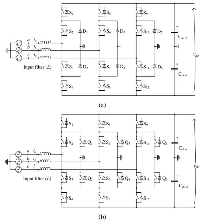
Fig. 8. Neutral-point-clamped ac-dc converters: (a) the conventional NPC converter, where the clamping diodes could be replaced with active semiconductors in the ANPC converter; (b) the active neutral point clamped (ANPC) converter.
