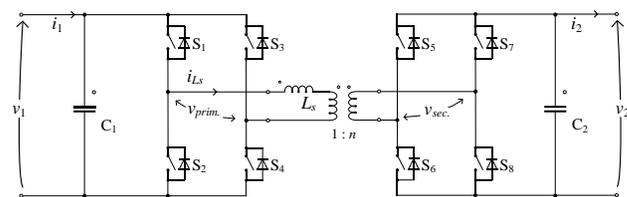
Fig. 10. Dual-active bridge converter, where the leakage inductance ( $L_s$ ) is used as an energy storage element, and two active bridges are used to control the power flow between  $v_1$  and  $v_2$ .
