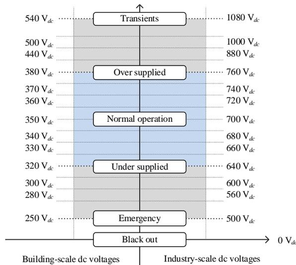
Fig. 5. Voltage levels and limits for LVDC electrical installations [65].
