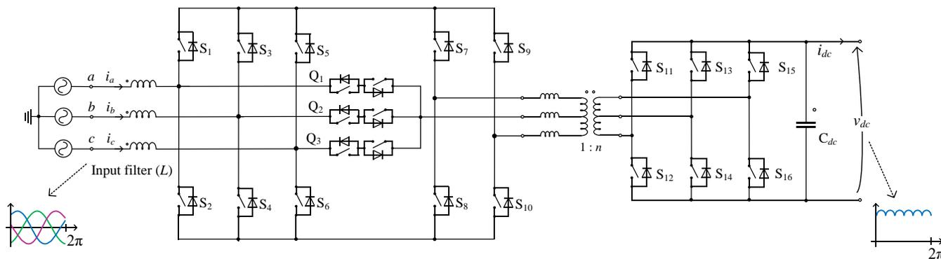
Fig. 16. Power circuit of the quasi-single-stage i-AFE converter based on the T-type and full-bridge converter used to allow operation with a three-phase transformer.
