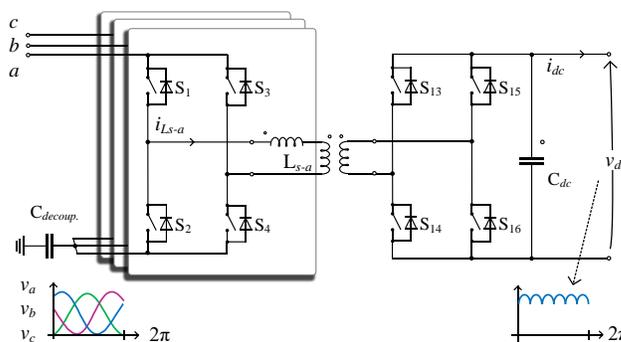
Fig. 21. Power circuits of the three-phase single-stage cascaded full-bridge i-AFE converter.
