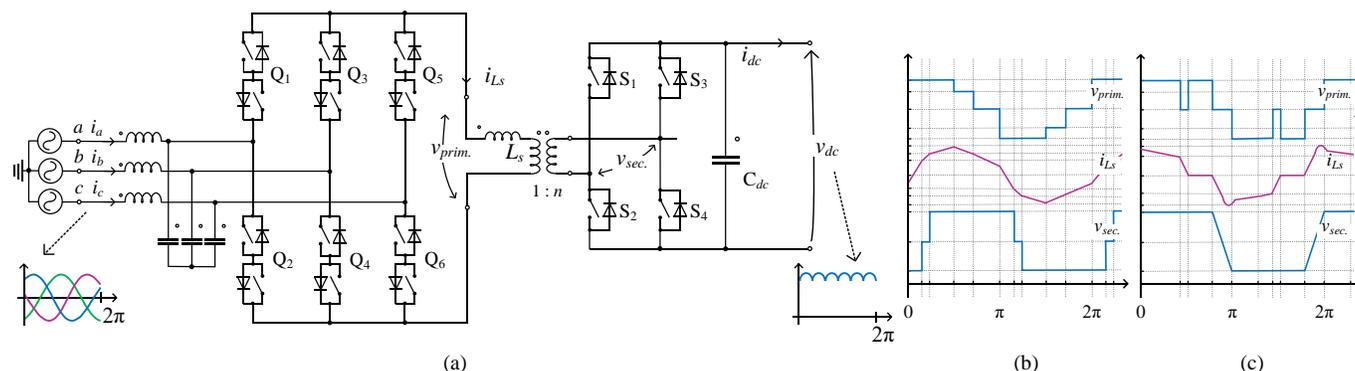
Fig. 20. Power circuit and examples of modulation strategies of the matrix-based dual-active bridge:(a) the power circuit where the first active bridge of the conventional DAB is replaced by the matrix converter with fully controlled semiconductors ( $Q_x$ ); (b) the Type-A pattern to modulate the matrix-based DAB converter; (c) a quasi-resonant modulation.
