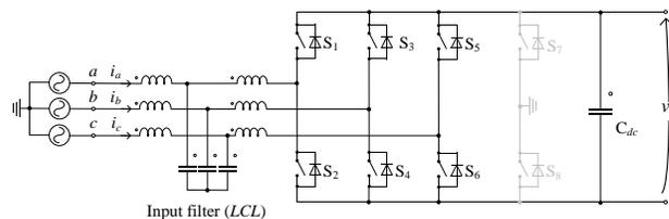
Fig. 7. Three-phase 2L-VSC PFC. Three-legs are used to connect to the ac grid with three-wire systems. In four-wire systems, an additional leg ( $S_7$ - $S_8$ ) is necessary to connect to the neutral point. For the ac side,  $LCL$  and  $L$  filters are possible.
