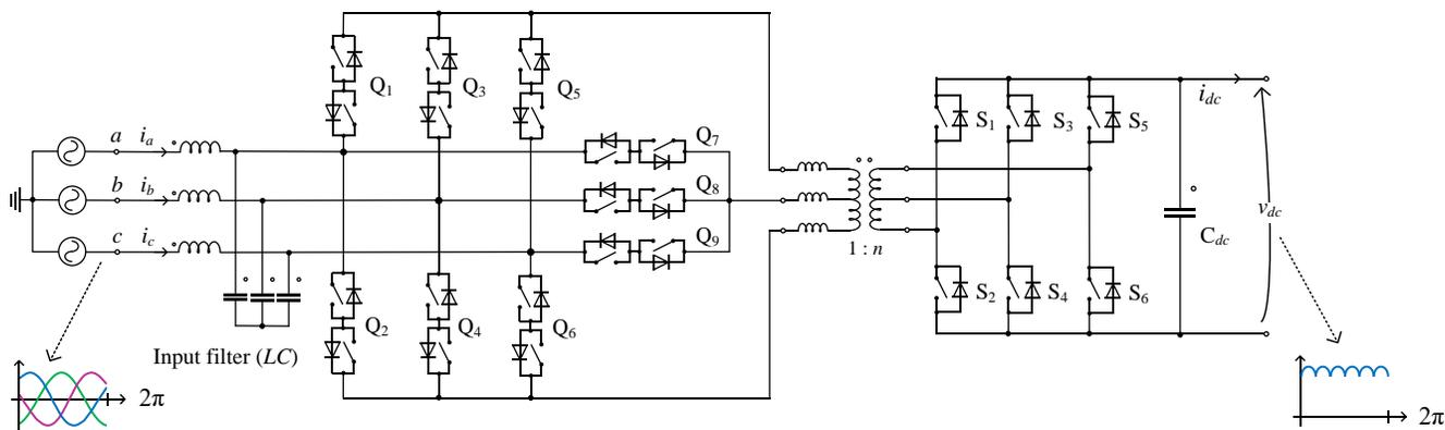
Fig. 23. Power circuits of the three-phase single-stage T-type NPC i-AFE converter.
