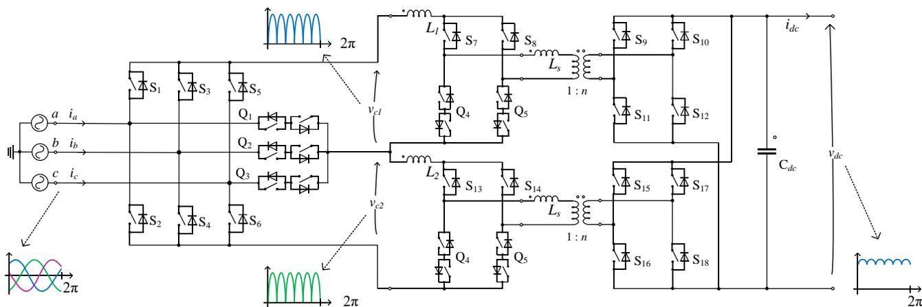
Fig. 18. Power circuit of an unfolded quasi-single-stage i-AFE converter based on the T-type and current-fed dual-active bridge.
