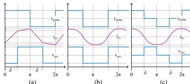
Fig. 13. Comparison of non-resonant and resonant dual-active bridge converters: (a) non-resonant DAB converter based on phase-shift modulation; (b) resonant dual-active bridge based on two-level voltages; (c) resonant dual-active bridge based on three-level voltages.
