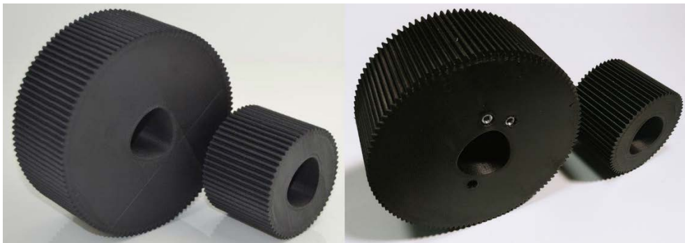
Figure 1: Test Samples. Polymer gears printed out of PEEK CFR 450 (left) and Onyx (right)
