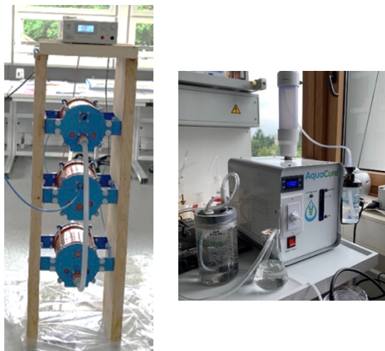
Fig. 4: The commercially available electrolyzers in the market to generate Brown's gas.
