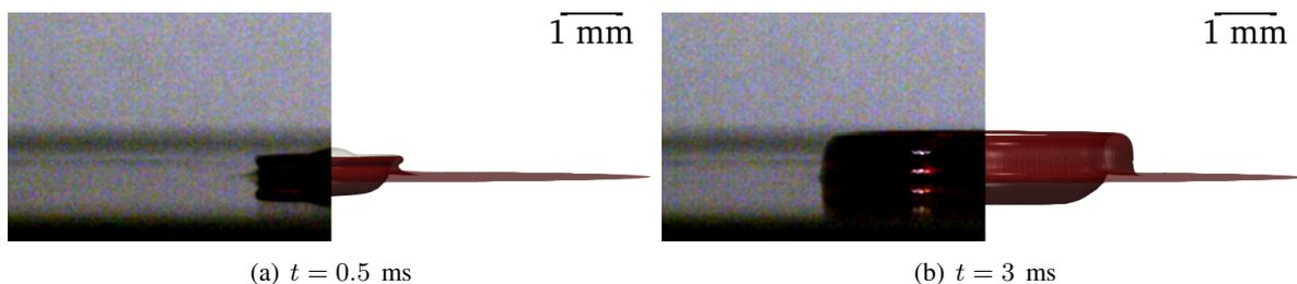
Figure 1: Recordings from the experiments (left) and simulations results (right). Water film is colored maroon and the oil drop is gray.
