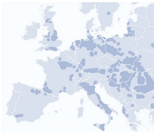
Figure 1: Distribution of existing oil/gas wells in Central and Western Europe as potential for HT-ATES (adapted from Pawlewicz 1997)
