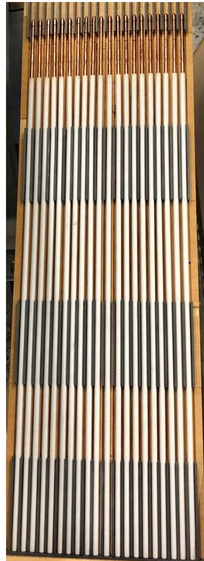
24 Mo/Cu upper electrodes partially coated by ZrO 2 (200 μm) OD 7.75 mm in coated region
