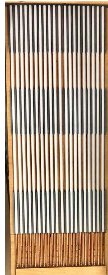
24 Mo/Cu lower electrodes partially coated by ZrO 2 (200 μm) OD 7.75 mm in coated region
