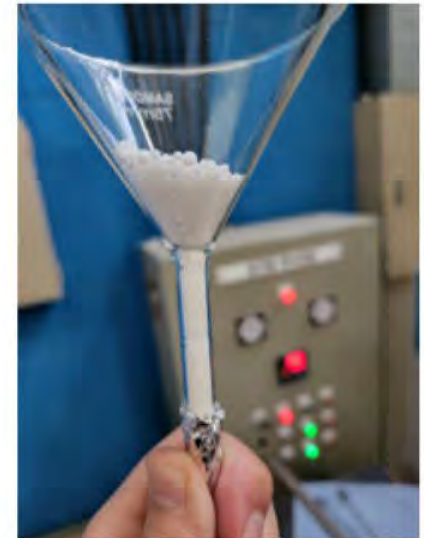
<Particle loaded into cladding>
