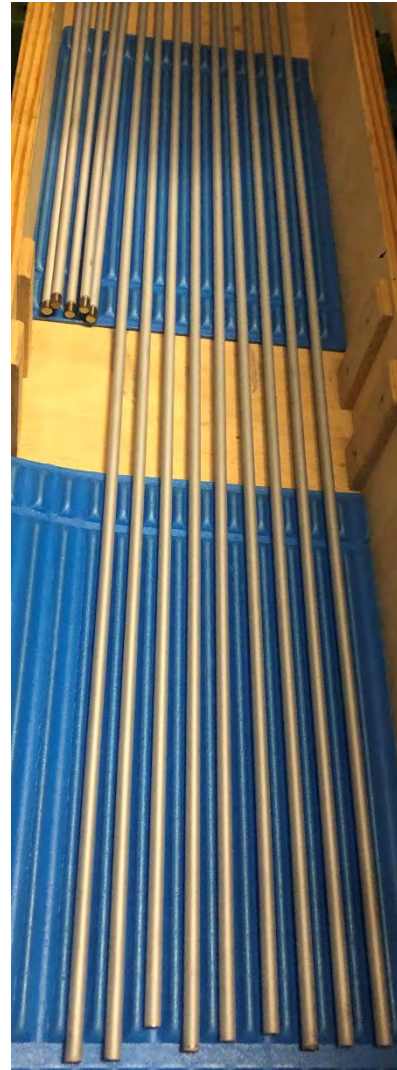
corner rods and tubes (OD 6 mm) PVD coated with Cr (10 μm)
