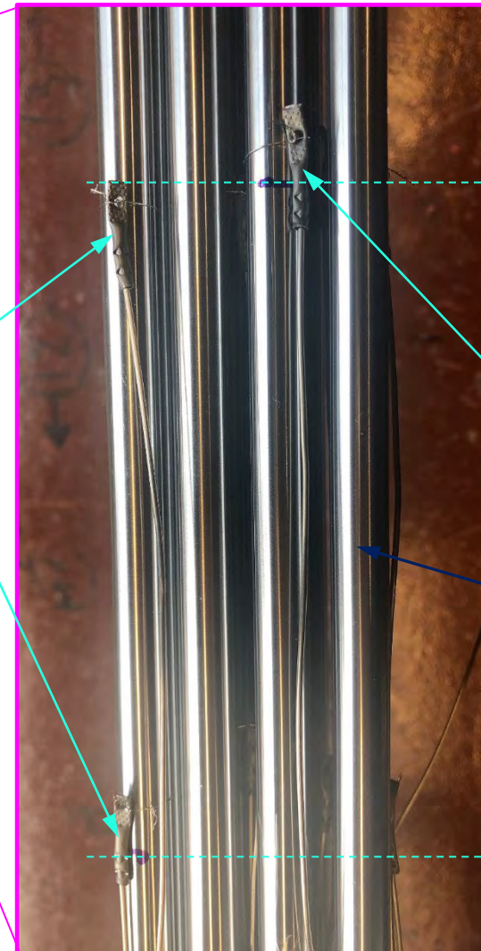
sheathed Ni/CrNi thermocouples attached to cladding surface with Pt/Rh wire wrapped around the rod
