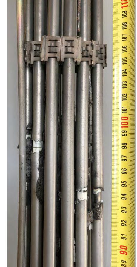
QUENCH-19 bundle post-test
