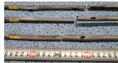
<Left: Strain fields measurements in 3D scanner, Right: bursted fuel rods held by a ceramic spacer grid>
