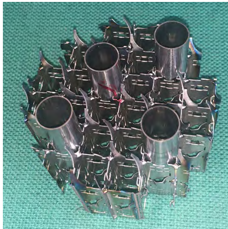
eroded grid spacer pitch 12.6 mm
