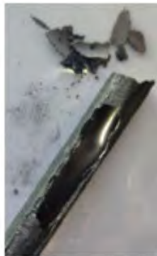
<Surface morphology of Cr-coated cladding after high temperature steam exposure>
