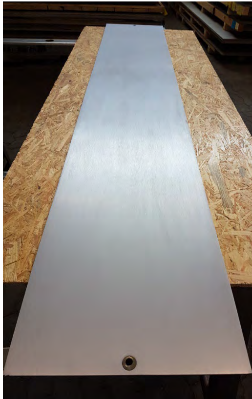
Zr sheet (thickness 3 mm) PVD coated at OERLIKON BALZERS GmbH with Cr (10 \mu\text{m} , X-ray measured) at one side
