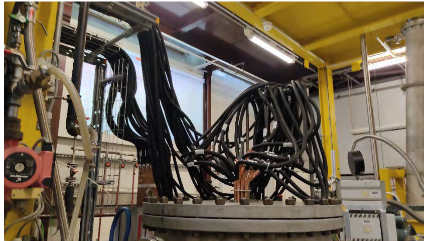
Electrical connections for current measurements at each rod
