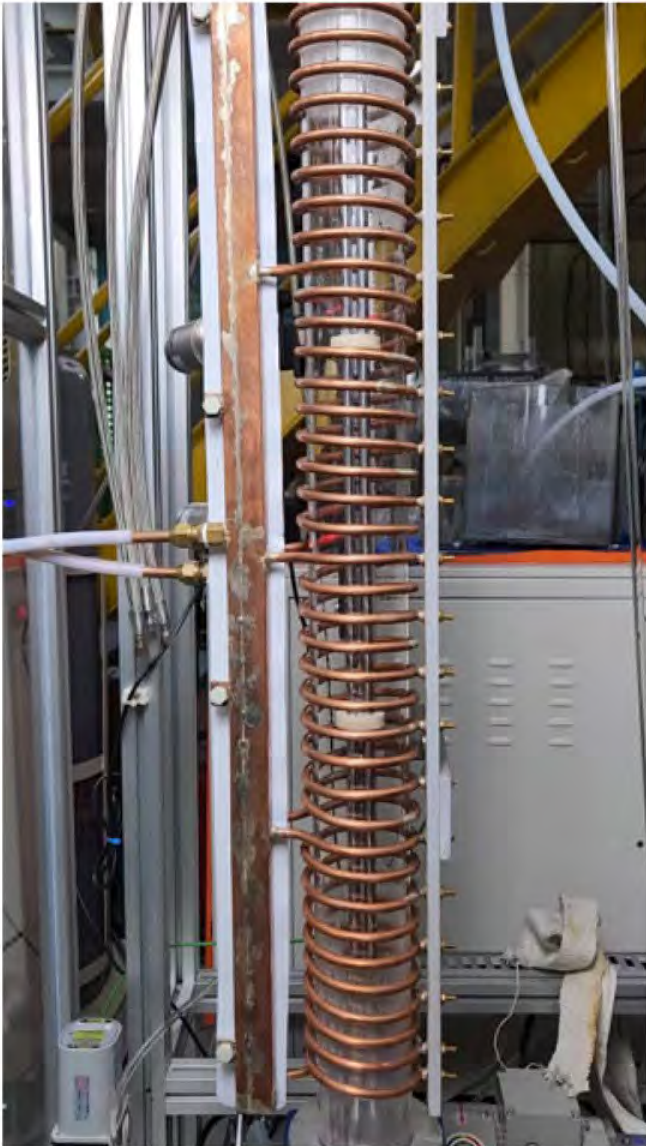
<Cr coated cladding (Zr-Cr-1.1Nb ) high temperature exposure test>
