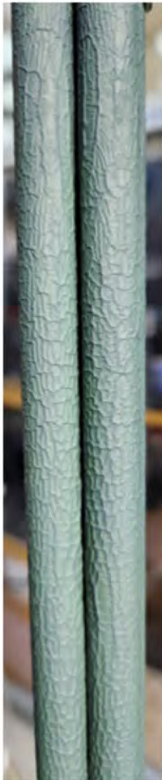
<Surface morphology of Cr-coated cladding after high temperature steam exposure>
