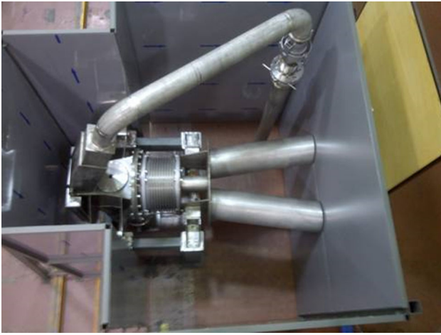
Fig. 27 Target System prototype installed at ENEA DRP laboratory
