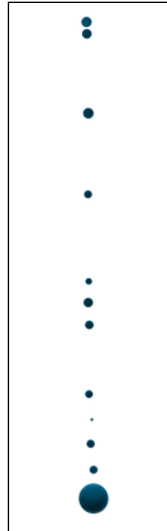
Figure 6. Satellite drops in inkjet printing. The main droplet is followed by multiple smaller droplets.
