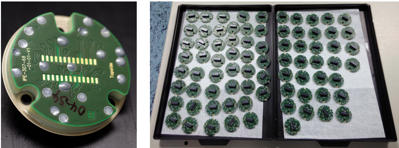
(a) Stack after dispensing the acoustic backing material.
