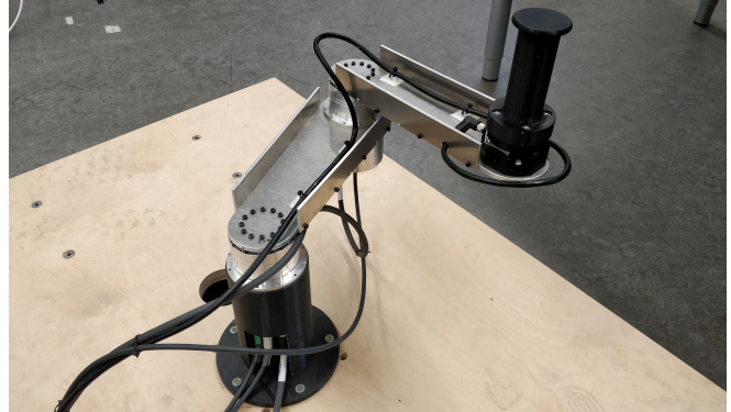
Fig. 9: A planar manipulator with 2 joints in SCARA configuration was used for the evaluation on real hardware.
