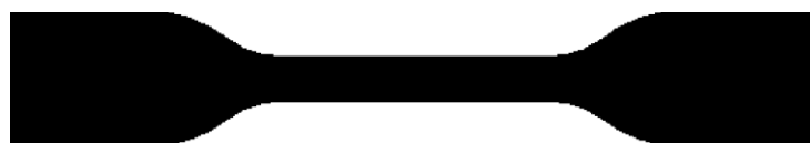
Figure 43: BMP template for the inkjet printing of specimens for mechanical measurements via tensile test.
