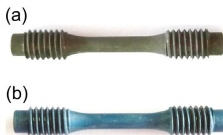
Fig. 11. LCF specimens of EUROFER for additional experiments: (a) after annealing with ceramic pebbles in vacuum for 64 days, (b) after annealing in a purge gas atmosphere for 64 days.
