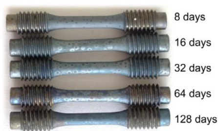
Fig. 1. LCF specimens of EUROFER after annealing for different durations together with ceramic pebbles in a purge gas atmosphere.
