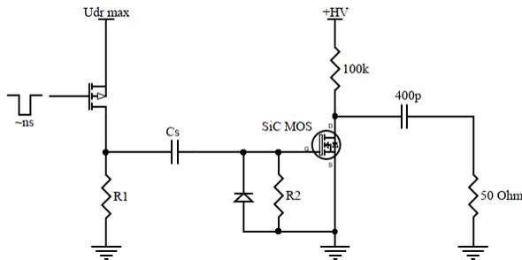
Figure 1: Schematic of super boosting setup.
