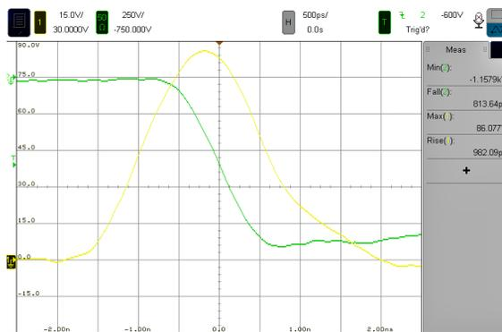
Figure 4: Gate-source (yellow) and load voltage (green) with 280 V driver and U<sub>ds</sub> = 1.3 kV; measurements are influenced by scope and probe BW limitation (1 GHz and 700 MHz respectively).
