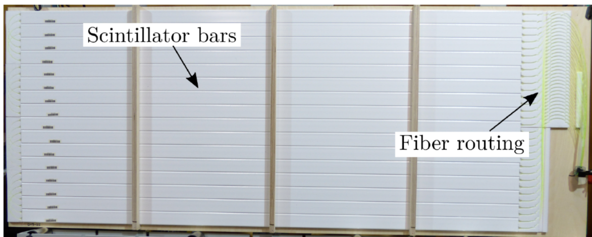
Figure 3.7.: Picture of the inside of one scintillator panel comprised of 16 scintillator bars. The wavelength shifting fibers are of same length in order to guarantee similar light propagation in each part of the scintillator panel. The fiber bundle is then connected to the SiPM. Picture taken from [99].
