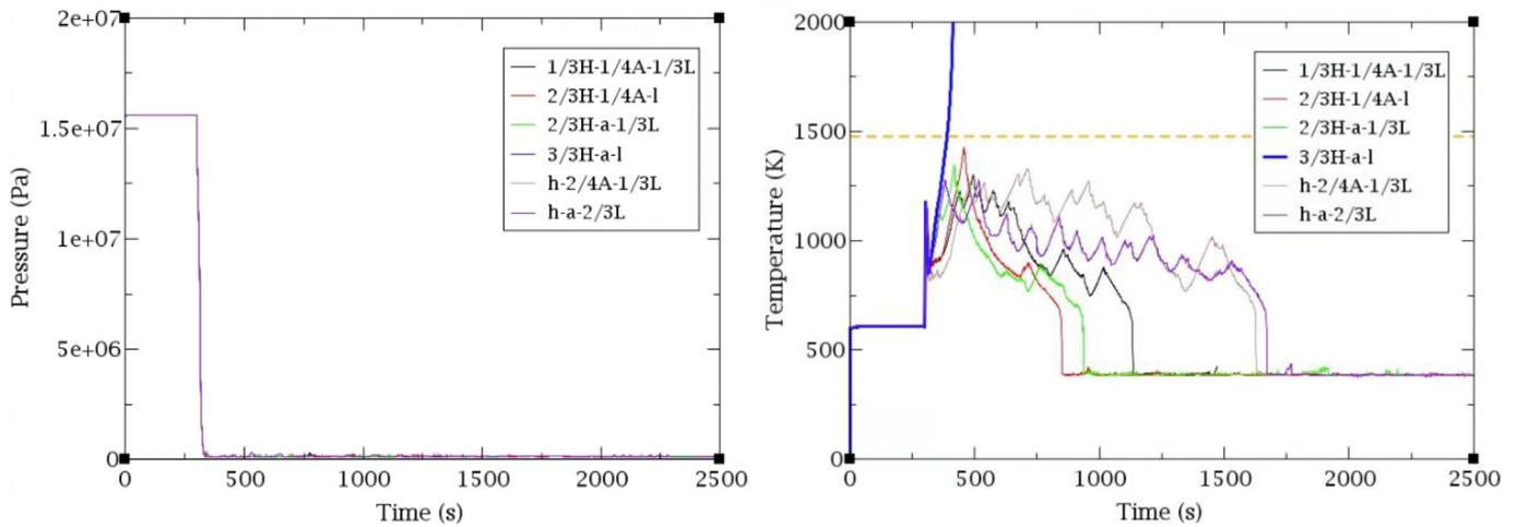
Fig. 14. RCS Pressure (left) and PCT (right); LBLECA DEGB sequences.
