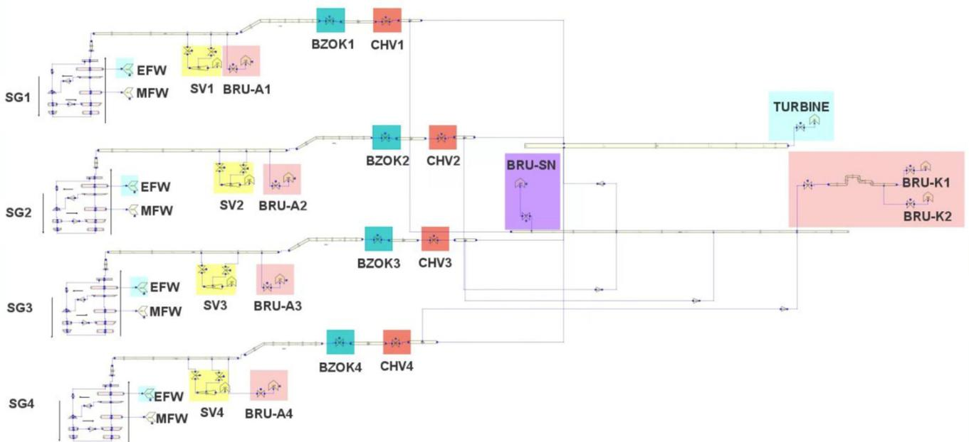
**Fig. 5.** Secondary side of VVER-1000/V320 TRACE TH model.
