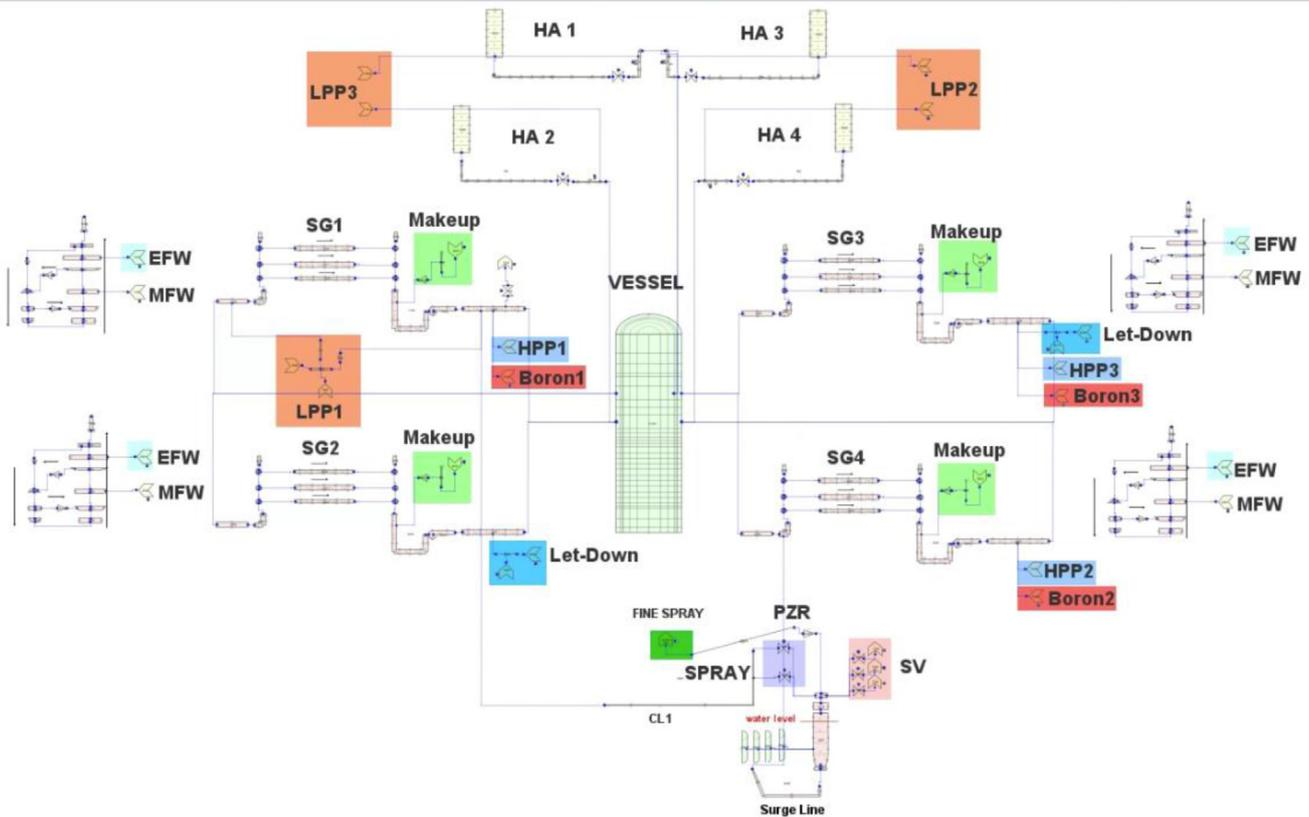
Fig. 4. Primary side of VVER-1000/V320 TRACE TH model.
