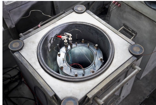
Large canister in EV+ ARC
