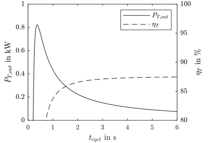
Fig. 7: Tower power and efficiency as a function of cycle time
