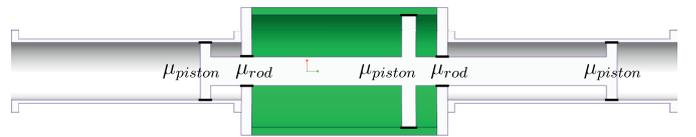
Fig. 4: Friction contacts working cylinder
