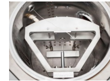
Nail penetration test in ARC
