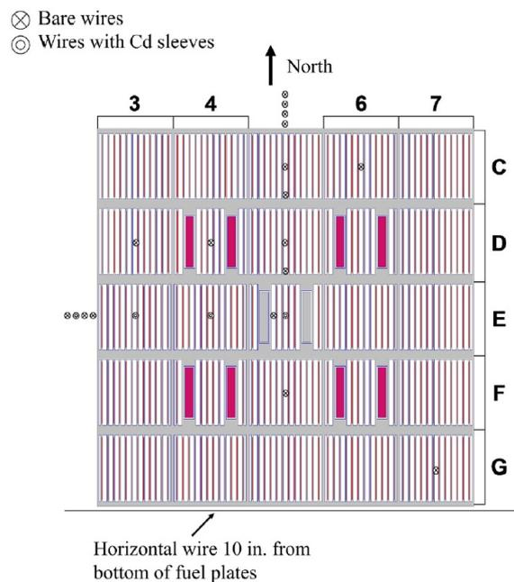
Fig. 3. Radial position of cobalt wires for thermal flux measures, [10]
