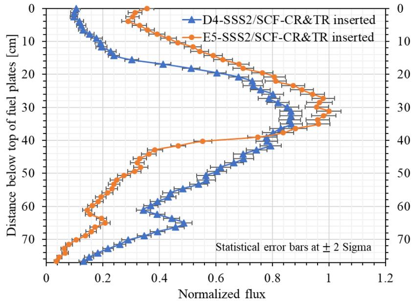
Fig. 8. Thermal flux normalised simulation, control and transient rods (CT & TR) inserted
