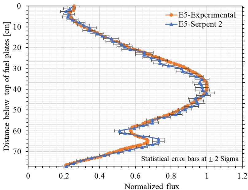
Fig. 5. Comparison of thermal flux detectors at location E5
