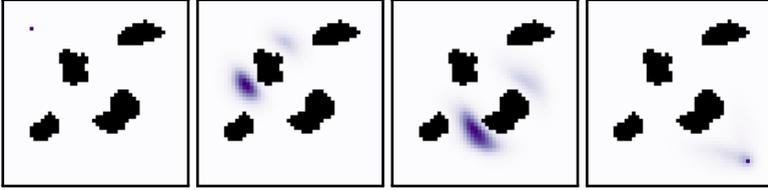
(b) Simulation of the policy derived from value function. High penalties for obstacle collision lead to multimodal trajectory prediction.
