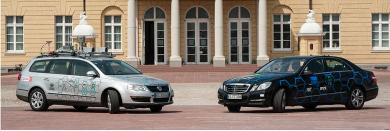
Figure 6.1.: Experimental vehicles of the Institute of Measurement and Control Systems. AnnieWay (left) used in the DARPA Urban Challenge [80] and BerthaOne (right) used in preparation of the Bertha Benz Memorial Drive [184].
