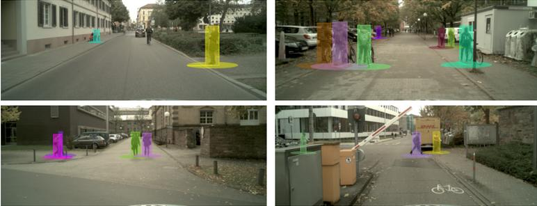
Figure 6.7.: Pedestrians annotations in images. Information includes the enclosing bounding box, position w.r.t. the vehicle and occlusion.
