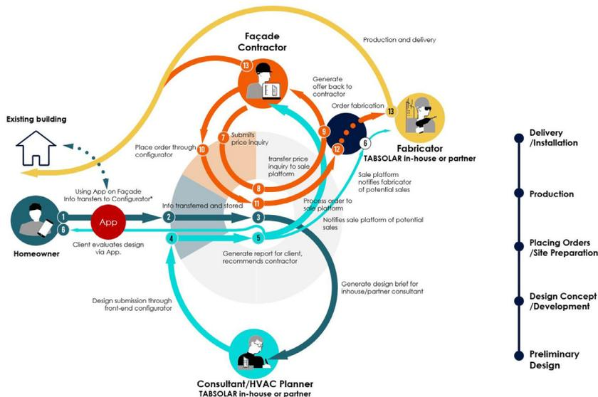
Fig. 4. Workflow of the TABSOLAR® use case building renovation.
