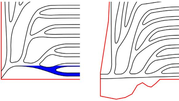
Fig. 5. Creation of FracTherm<sup>®</sup> channel design: rectangular area leads to negative channel slopes and thus remaining fluid (left), adjusted boundary form “forces” algorithm to create positive channels slopes in order to ensure full emptying (right).
