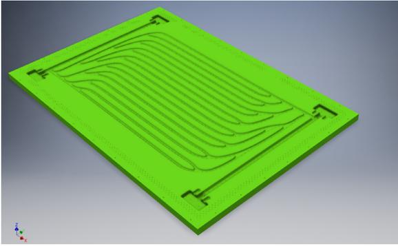
Fig. 11. CAD drawing of mold for membrane vacuum deep-drawing process (1683 mm x 1040 mm).
