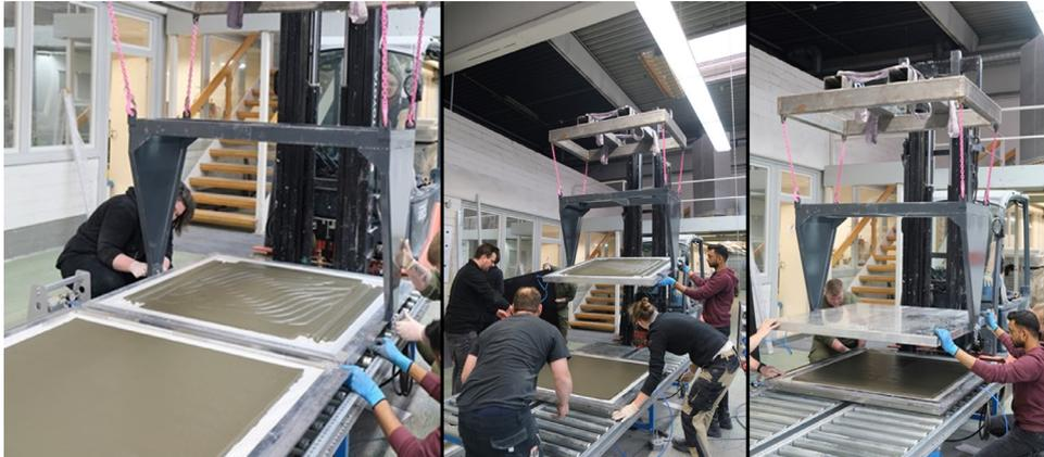
**Fig. 13.** Small-scale sample plant: molds prepared to be joined together (left), turning the deep-drawn formwork (center), positioning before joining (right).
