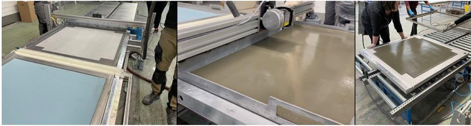
**Fig. 12.** Small-scale sample plant: molds and material application (left), application of fresh concrete (center), fresh concrete layer prepared for deep-drawing (right).
