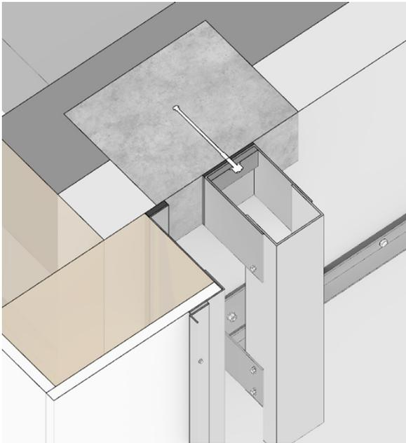
Fig. 24. Concrete posts as a foundation for the substructure.
