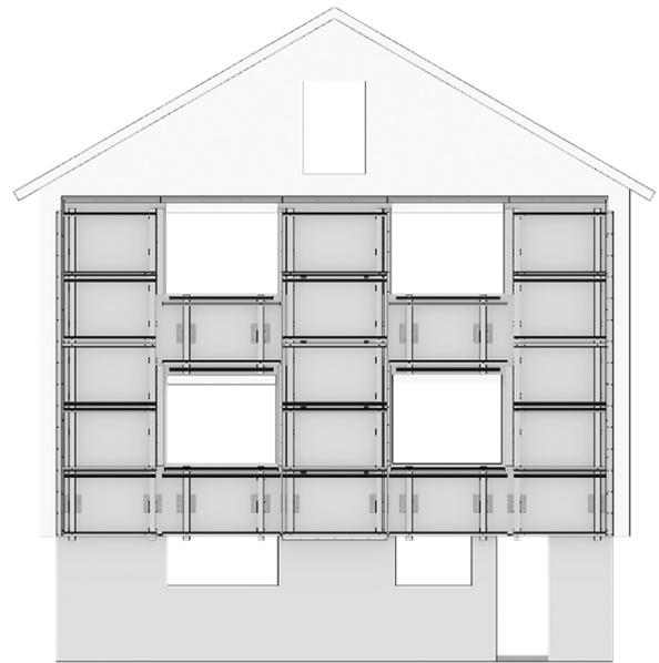
Fig. 25. Layout of the vertical profiles and traverses.
