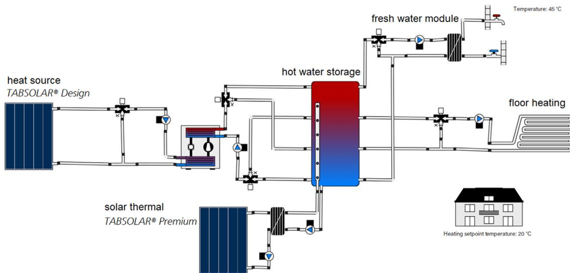
Fig. 20. Hydraulics of the simulated system.
