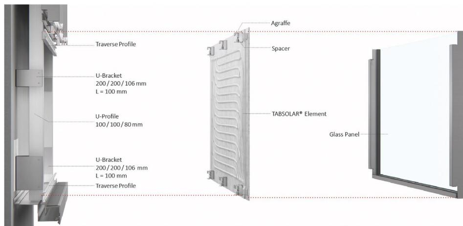
Fig. 26. Exploded view of the TABSOLAR® demonstration façade structure.
