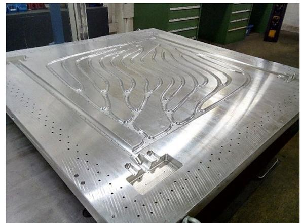
Fig. 10. Milled mold for membrane vacuum deep-drawing process (1040 mm x 1040 mm).
