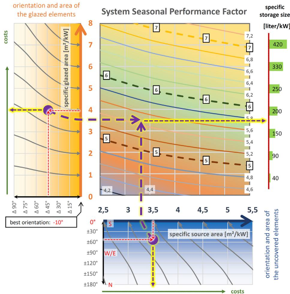
Fig. 21. System design map with sample configuration.
