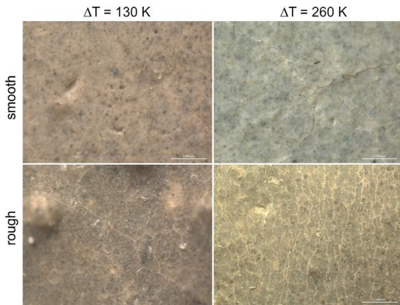
Fig. 17. Surface cracking due to thermal shock (light microscope).
