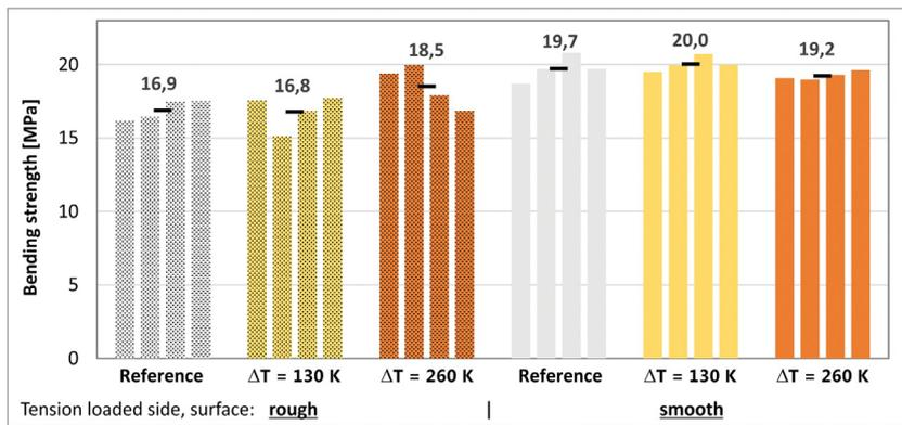
Fig. 19. Bending strengths of reference and quenched specimens (4 samples each and mean value).
