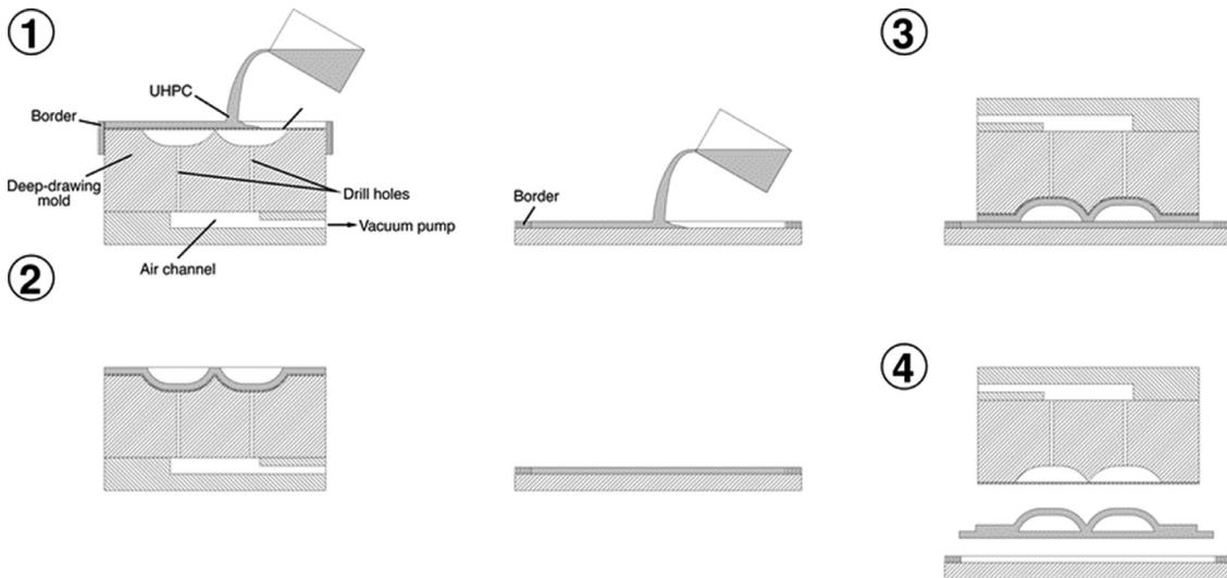
Fig. 7. Basic principle of membrane vacuum deep-drawing process (details and further developments not shown).
