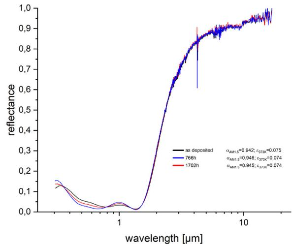
**Fig. 16.** Reflectance vs. wavelength of small UHPC sample with spectrally selective coating between lacquer coats.
