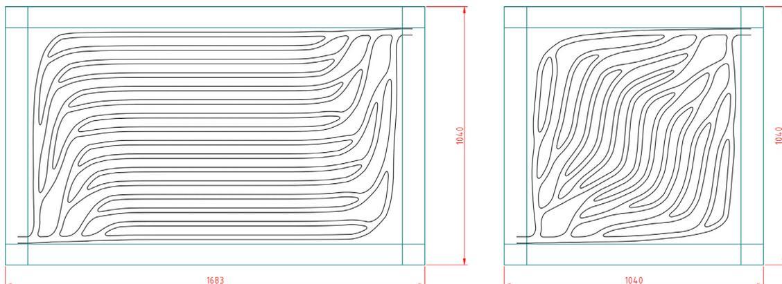
Fig. 6. FracTherm<sup>®</sup> channel designs for large TABSOLAR<sup>®</sup> element (left, 1683 mm x 1040 mm) and for small TABSOLAR<sup>®</sup> sample (right, 1040 mm x 1040 mm) with border areas for agraffes and collecting channels.
