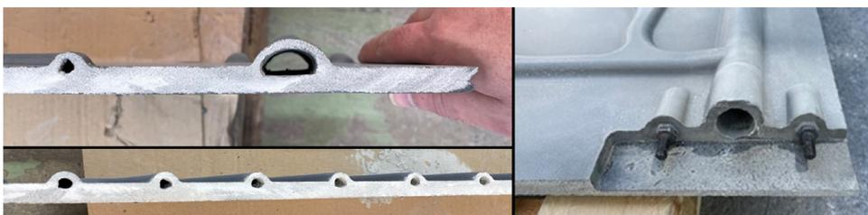
**Fig. 15.** TABSOLAR® samples: cross sections (left top and bottom), cylindrical bush for hydraulic connectors (right).
