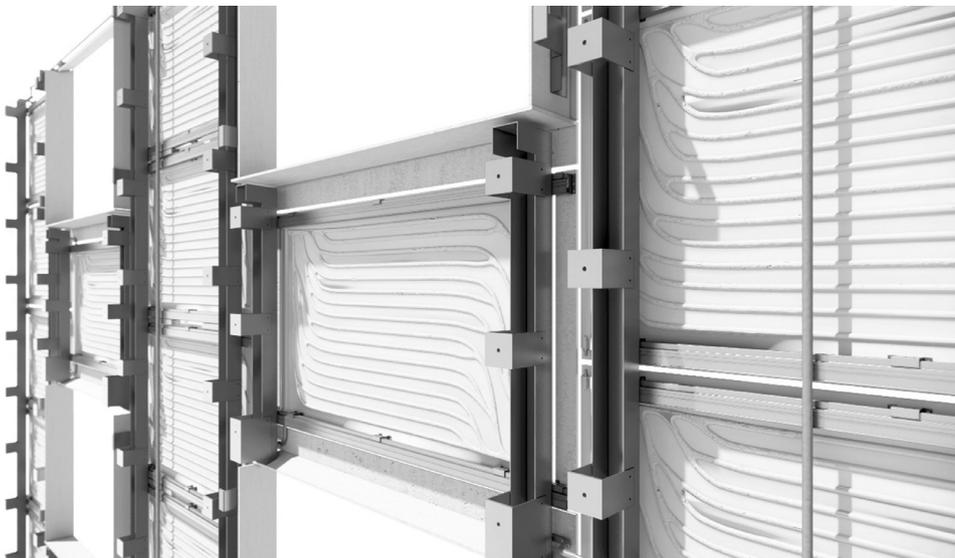
Fig. 27. Rear view of the structure with integrated piping.
