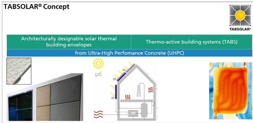
Fig. 1. TABSOLAR® concept: novel thermal components for building envelopes and interiors.
