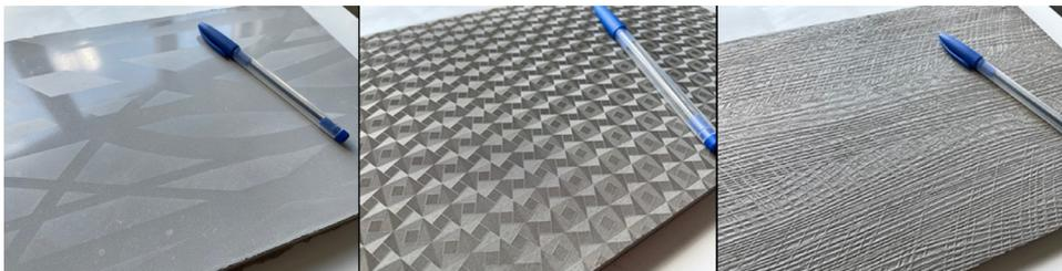
Fig. 9. Different surfaces of casted UHPC: matt/glossy (left), relief/microstructure (center), wood texture (right).
