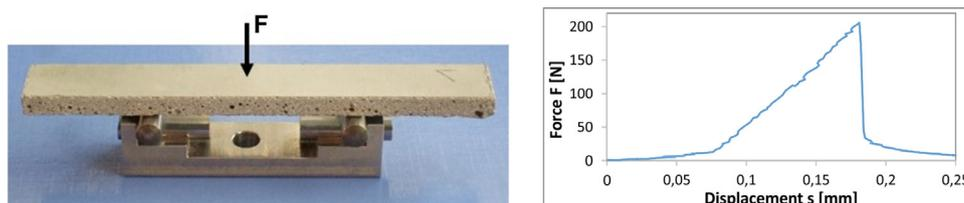
Fig. 18. UHPC specimen and device for three-point bending test (left) and a typical force-displacement curve (right).
