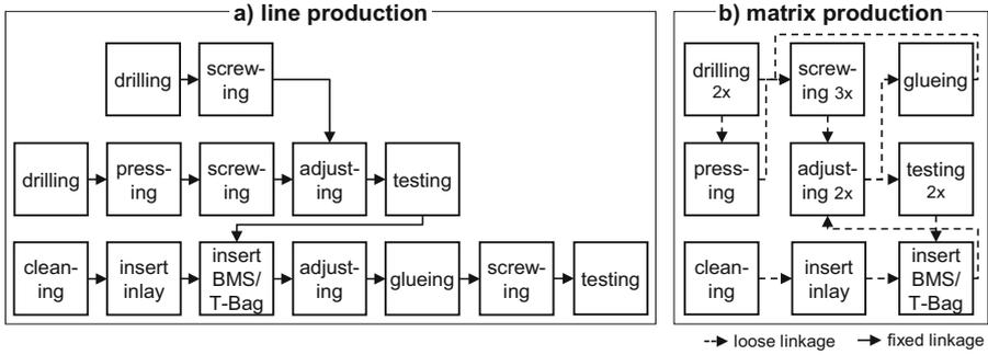
Fig. 3. Production process of line and matrix production
