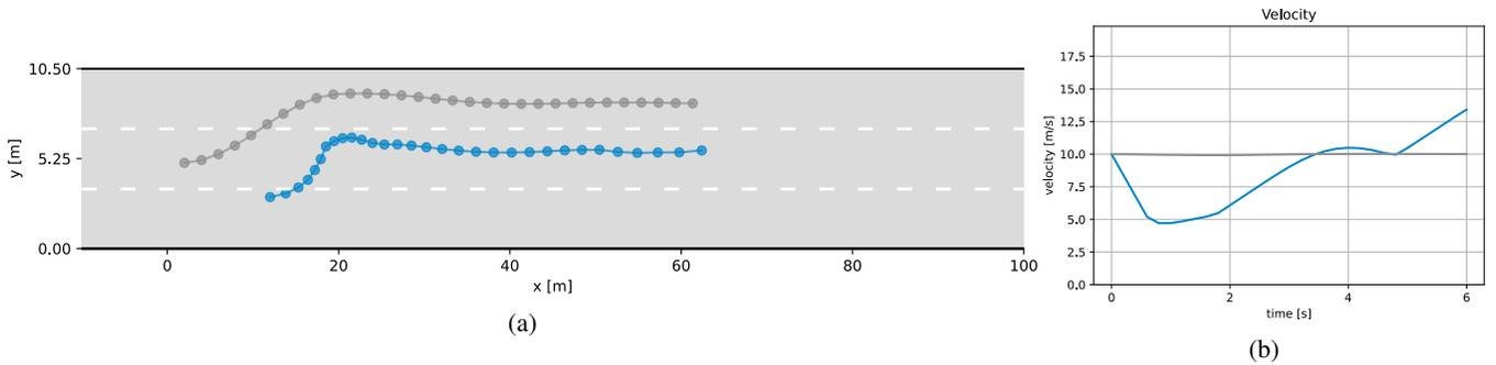
Fig. 3: To push the follower to the leftmost lane, the leader brakes harshly and steers to the left.
