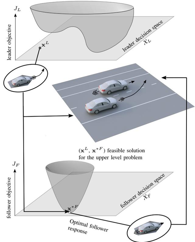
Fig. 1: Illustrated is the structure of a Stackelberg game modeled as a bi-level optimization problem. Here, the follower optimizes its objective function as a response to the given actions of the leader.
