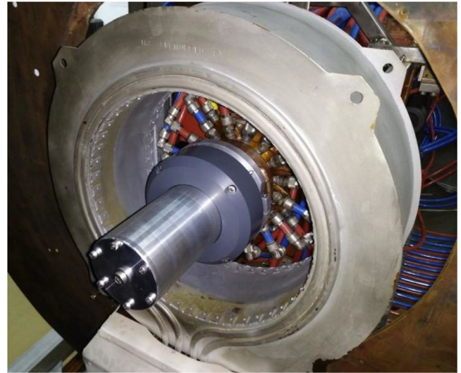
Fig. 9. The SX3 AF-MPDT thruster of the IRS within its large applied-field coil [43].
