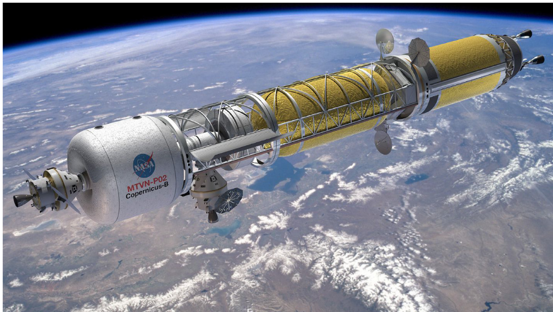
Fig. 8. A Mars Transfer Vehicle of the Mars Design Reference Mission 5.0 concept study of NASA [40].
