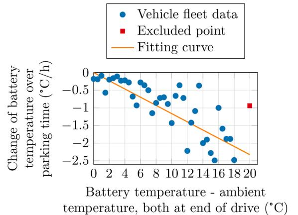
**Fig. 5.** Curve fitting of the battery temperature change of a parked vehicle using vehicle fleet data. Each point represents the average value of all observed rates (y-axis) within buckets of 0.5 °C for the corresponding difference in temperatures at end of drive (x-axis).
