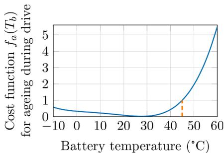
**Fig. 4.** Cost function for temperature dependent battery ageing based on [8], after scaling to 1 at 45 °C as marked by the dashed line.
