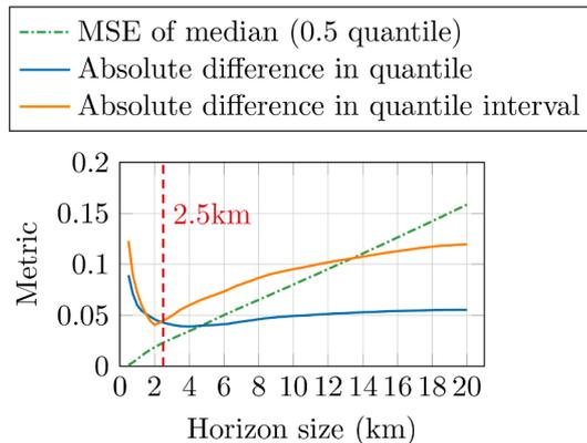
Fig. 2. Metrics of the QCNN on test data as given in [22], with better performance for lower values and calculated for different horizon sizes. The metrics include the Mean Squared Error (MSE) of the median prediction and the occurrence of true values within the predicted quantile and quantile interval. A dashed line marks the intersection of the two latter metrics.
