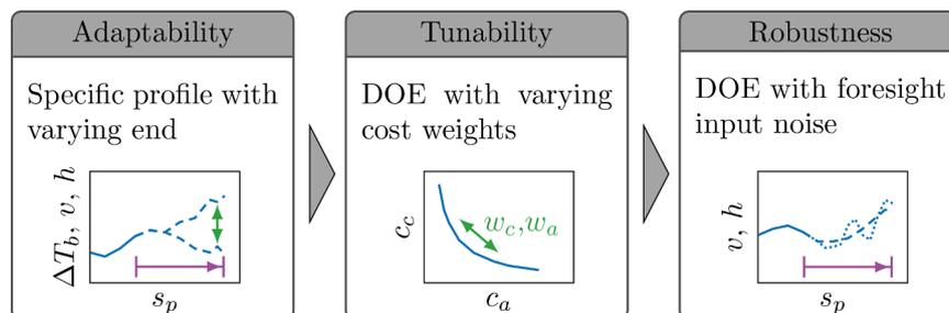
**Fig. 6.** The analysis of the developed predictive control includes the effect of variation of input foresight data (speed  $v$ , height  $h$ ) and cost weights (ageing  $w_a$ , cooling  $w_c$ ) on the predicted change in battery temperature  $T_b$  over the prediction horizon  $s_p$  and the resulting costs (ageing  $c_a$ , cooling  $c_c$ ). The DOE is shown in Table 1.
