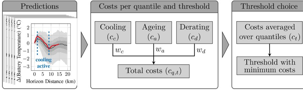
**Fig. 3.** Calculation steps leading from previously obtained predictions per threshold to the choice of a battery cooling threshold. The shown prediction example is taken from [22]. Costs are denoted by  $c$  and their cost weights by  $w$ .
