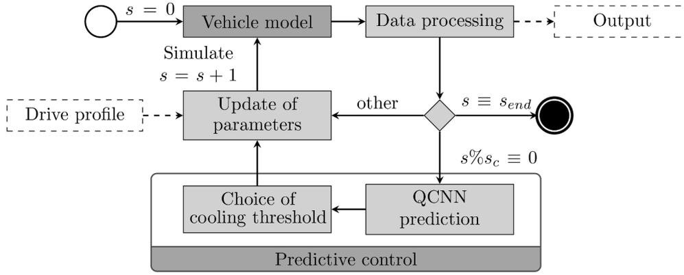
Fig. 1. Control framework including a vehicle model and a QCNN for battery temperature prediction. A predictive control is conducted each time when the driven distance  $s$  passed the control distance  $s_c$  and when the total distance  $s_{end}$  of the profile is not reached yet.
