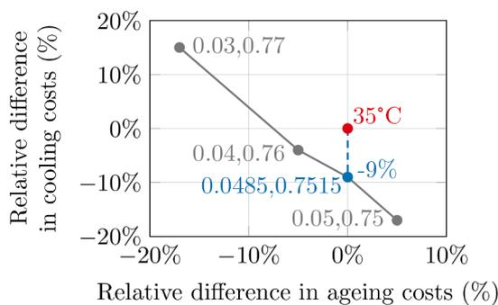
Fig. 9. Comparison of cooling costs and ageing costs with respect to the results with a fixed threshold of 35 °C. The weight set (0.0485,0.7515) shows a potential reduction of cooling costs by -9% with same ageing costs.
