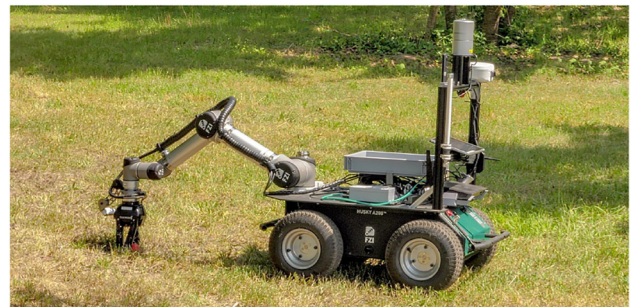
Figure 11: The modified Husky robot from FZI used during the test deployment is shown grabbing a golf ball representing a contaminant. The box on top is considered as the safe containment.
