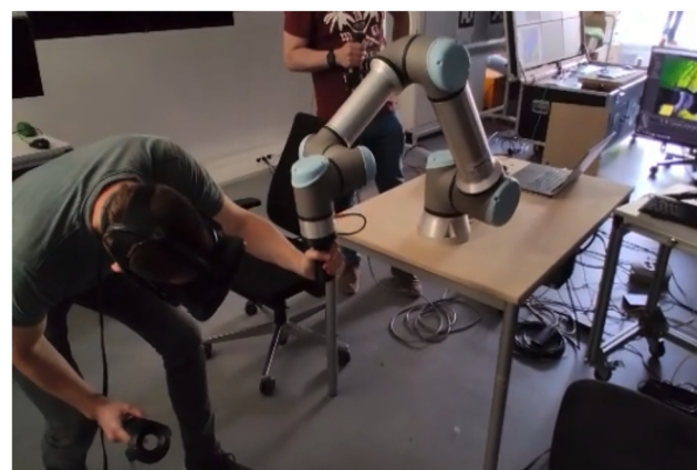
Figure 2: Physical setup of the control station. A teleoperator with a VR headset operates a haptic robot (UR16e) that is programmed with haptic rendering to behave like a remote UR5.
