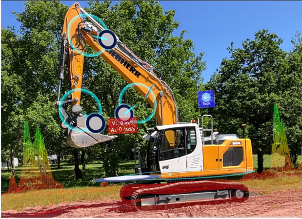
Figure 7: Live teleoperation of an excavator from Fraunhofer IOSB, a ROBDEKON partner, with an iPad. The excavator's joints can be controlled individually by spinning the markers in blue.
