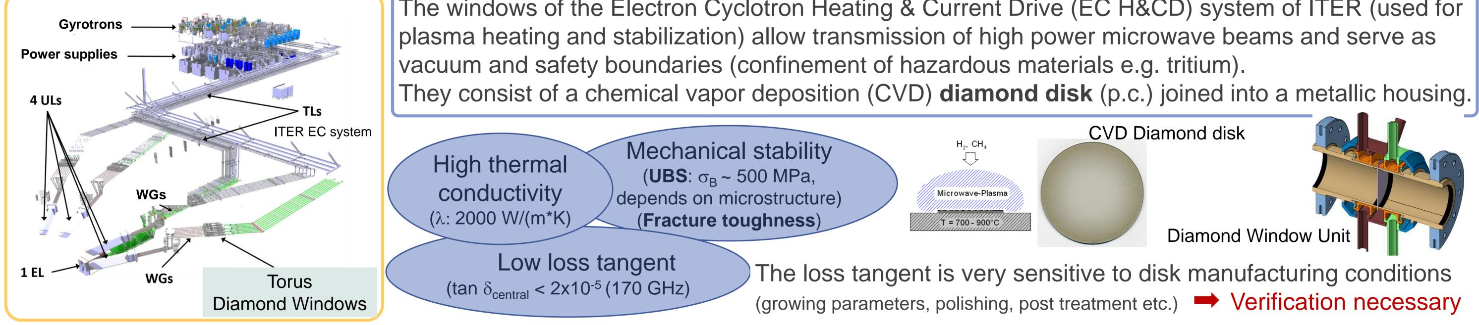
The windows of the Electron Cyclotron Heating & Current Drive (EC H&CD) system of ITER (used for
