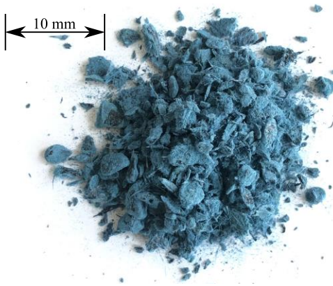
Figure 4-2: Manufactured PF-SGF40-LGF0 phenolic molding compound
