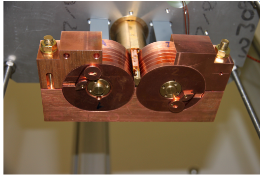
Figure 3.19.: Photograph of 2-period TGU explaining the SC coils, two cylindrical coil former and rectangular support structures [12].
