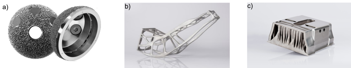
Figure 2.2: Example parts made by LPBF for different industrial applications; a) acetabular cup for hip implants made from Ti6Al4V, b) satellite bracket from AlSi10Mg, and c) mold with conformal cooling channels made from maraging steel
