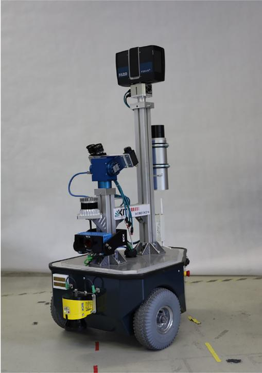
**Figure 2:** The completed autonomous exploration platform *GammaBot*.
