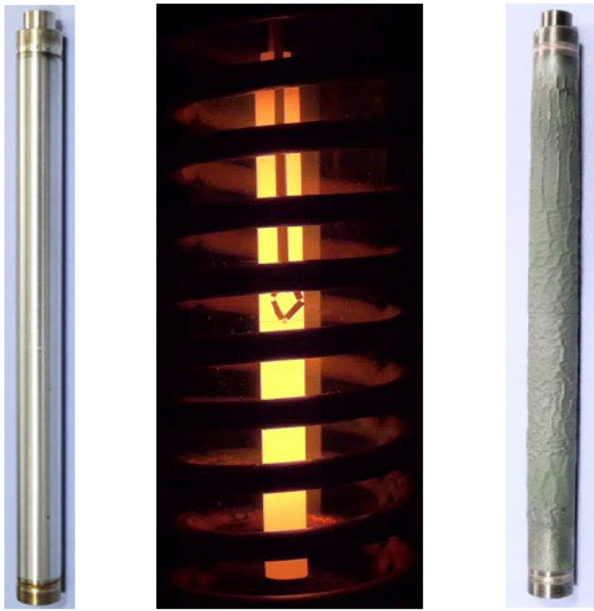
Fig. 3. Cr-coated samples before (left), during (mid), and after transient experiment up to >1500^{\circ}\text{C} .
