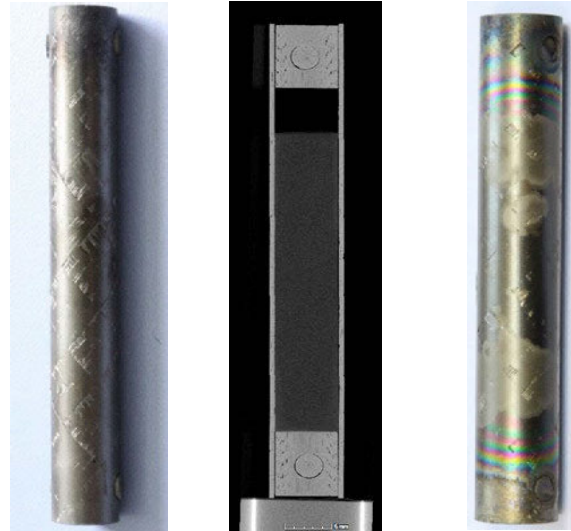
Fig. 10. SiC CMC samples as received (left), X-ray tomography showing end plugs and graphite core (mid), and after 1 hour steam oxidation at 1700^\circ\text{C} (right).
