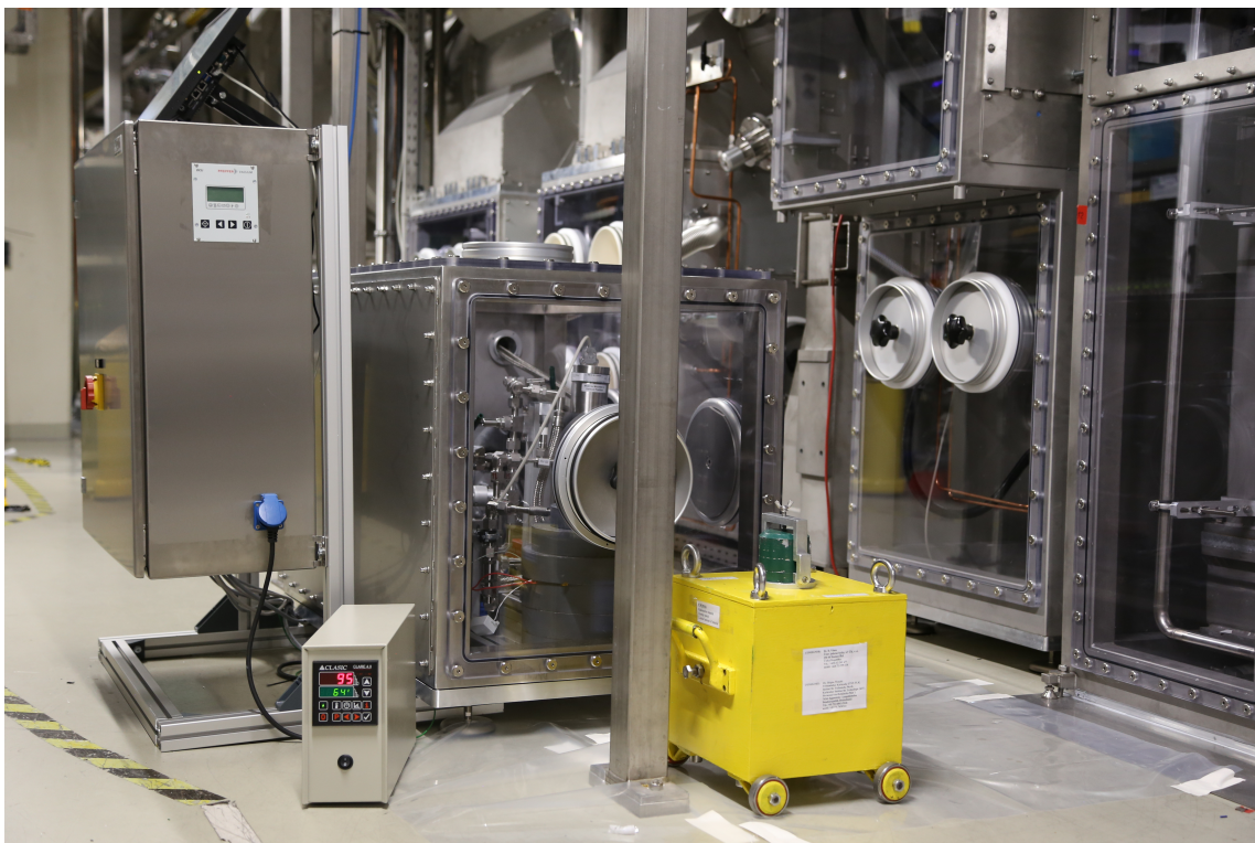
Figure 5. The ^{83}\text{Rb}/^{83\text{m}}\text{Kr} generator setup and yellow transport container. In the center, there is the 2 nd containment box with the generator setup located inside. Electricity power distribution cabinet and controller of the baking oven are on the left.
