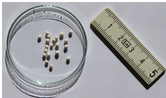
Figure 3. Picture of the ^{83}\text{Rb}/^{83\text{m}}\text{Kr} zeolite source, 20 spherules, total mass 0.15 g.
