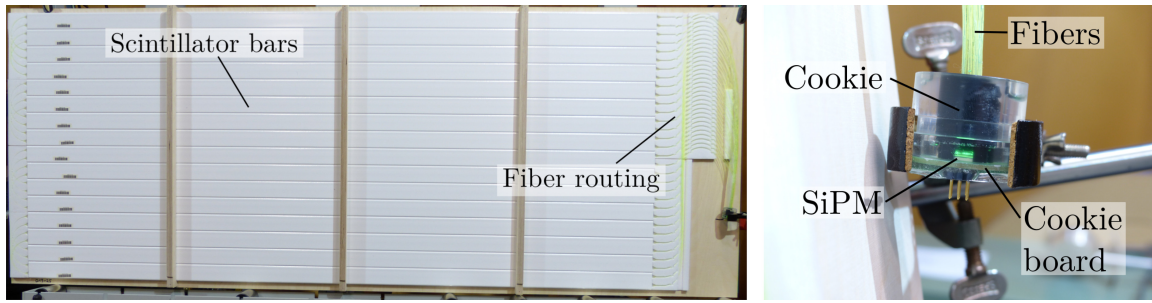
Figure 3.6.: Interior of the scintillator panel. Left: The 16 scintillator bars, mounted on the wooden base plate and held in place with wooden bars. The WLS fibers are routed through the scintillator bars and the polystyrene guides to one side of the detector, where they are bundled and connected to the Cookie. Right: Picture of the assembled cookie. The fibers are bundled and glued with optical cement to the cookie board [36]. On the cookie board are the SiPM and the temperature sensor. Pictures from [3].
