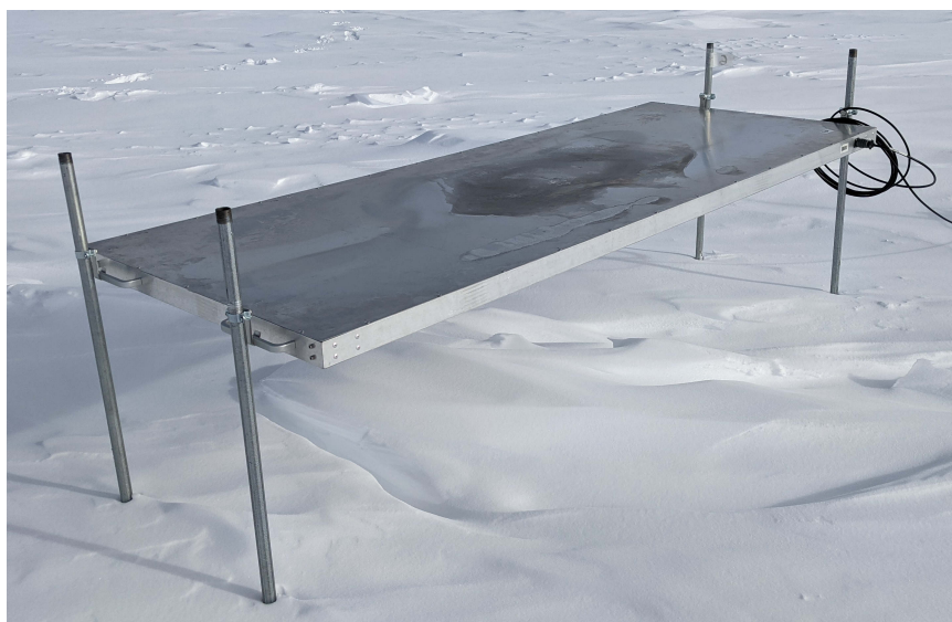
Figure 4.2.: Scintillator at the South Pole. The top of the mounting poles is threaded to allow an easy extension. This will be used to raise the detectors over the accumulating snow. It is not required for the station in Utah
