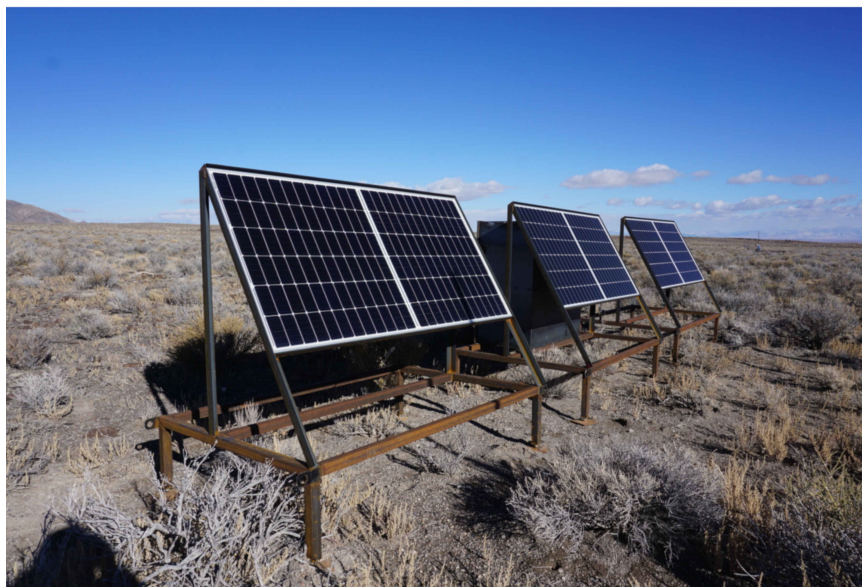
Figure A.8.: Pictures of the SAE station in the field. Top: Two scintillators of one of the station's arms being deployed. The scintillators use a version of the TA scintillator stands. The yellow straps are used to attach the scintillator stands to the helicopter. Bottom: Solar panels to power the SAE station. Three bifacial panels with an total power of around 1 kW are uses. Behind the middle panel, the battery box is visible. A picture of the center of the station can be found in Figure 8.2 [67].
