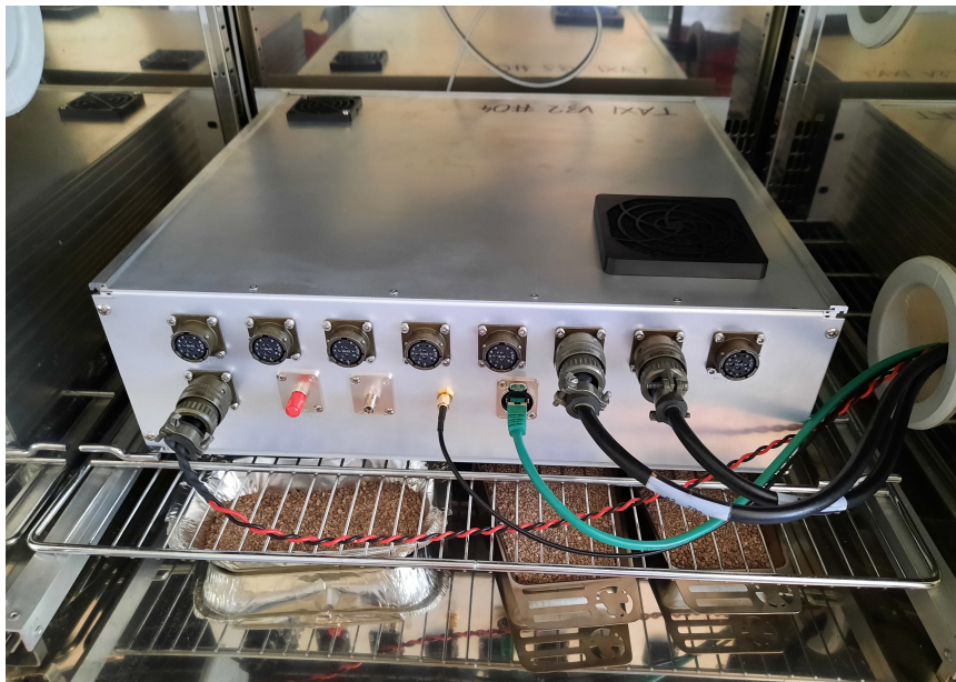
Figure 6.1.: TAXI in the temperature chamber. The chamber is used to test TAXI's heat sensitivity and the effectiveness of the fans at temperatures up to 50^{\circ}\text{C} . Two scintillator panels are connected to investigate the temperature dependence of the data corruption.
