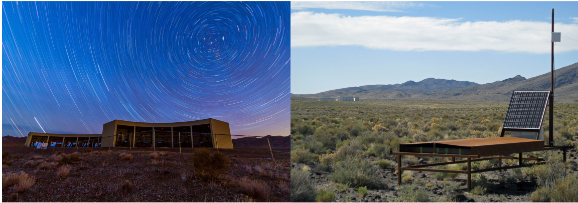
Figure 3.11.: Detectors of Telescope Array. Left: Picture of the Middle Drum fluorescence telescopes. The building on the left houses the TA telescopes, the building on the right the TALE telescopes. Credit: Ben Stokes, University of Utah. Right: Picture of a TALE scintillator in its housing, including solar panel and electronics box. In the Background, Middle Drum is visible.
