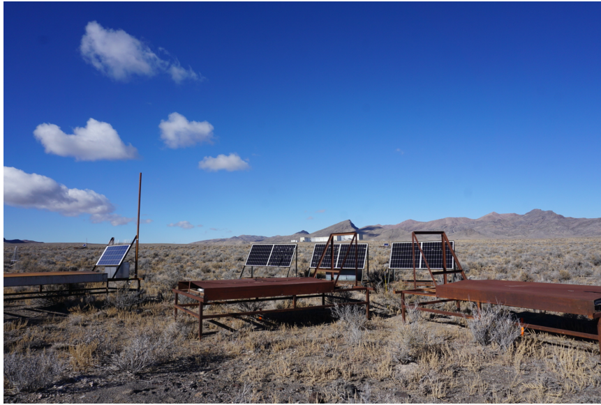
Figure 8.2.: Center of the deployed station on November 15, 2022. The central two scintillators of the SAE station are in the middle and on the right. Behind them are the solar panels to power the SAE station, on the left a TA scintillator and in the background the Middle Drum fluorescence detector [67].
