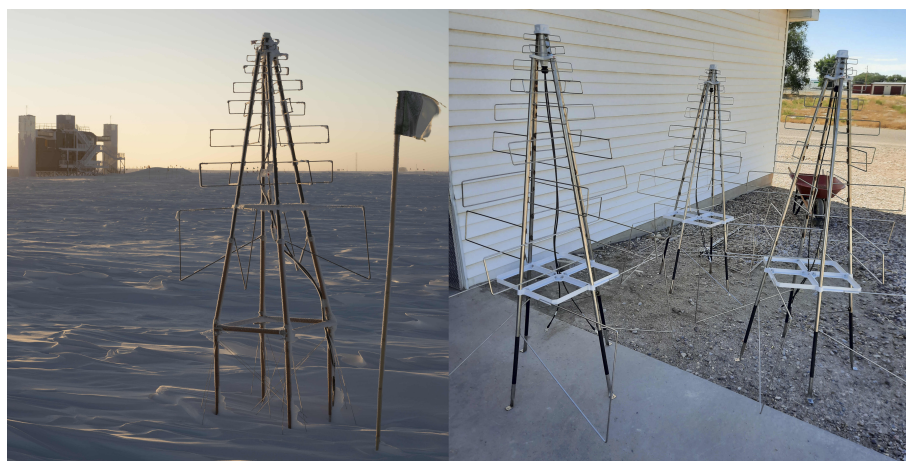
Figure 4.1.: Radio antennas at the South Pole and the Cosmic Ray Center. Left: Antenna at the South Pole with wooden structure. Right: Antennas at the CRC with their original metal feet.
