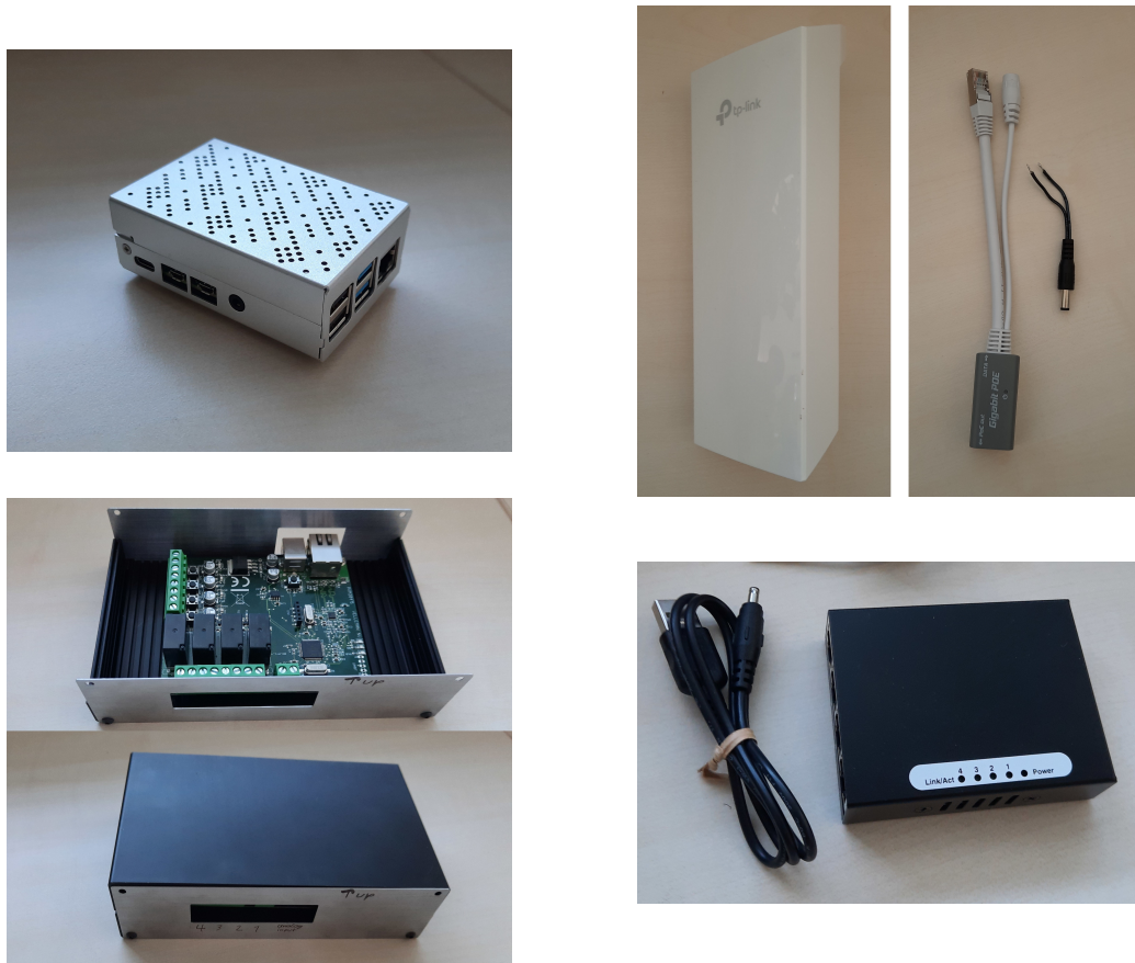
Figure 4.8.: New components of the DAQ system. Top left: Raspberry Pi. Via the Raspberry Pi, the communication with TAXI is established. It hosts the DHCP server for TAXI and directly collects the radio data. Top right: Outdoor WLAN antenna and access point to connect the station with the WLAN network from Middle Drum. The right side shows the power-over-Ethernet adapter to directly connect it to the 24 V supply. Bottom left: Ethernet relay card in its case. The case was built to protect the card, recycling scrap from the laboratory. Bottom right: Ethernet switch, used to connect the WLAN antenna with all the other components.
