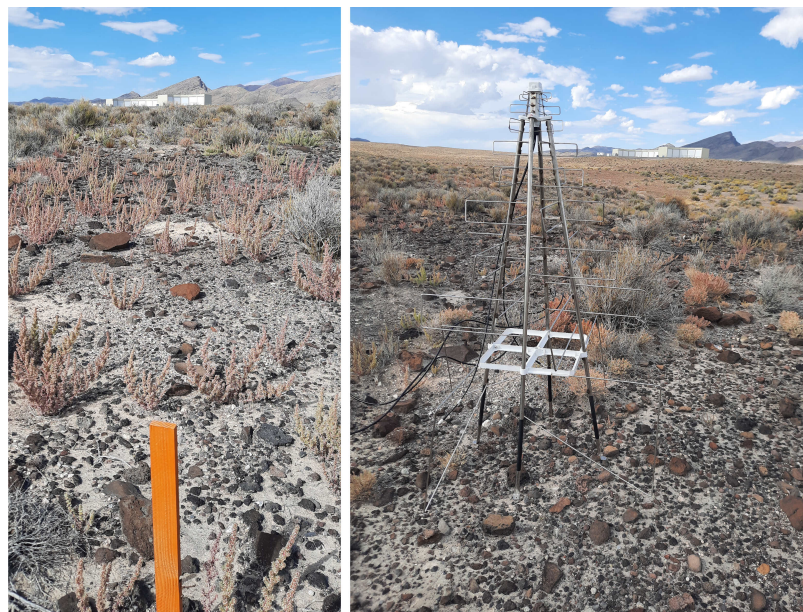
Figure 7.12.: Stake 5010 and antenna in field. Left: In the foreground stake 5010 and the terrain around it, in the background the Middle Drum fluorescence detector. Stake 5010 will be close to the center of the SAE station. Right: Antenna set up for the background measurement. On polarization is directed towards the fluorescence telescope.
