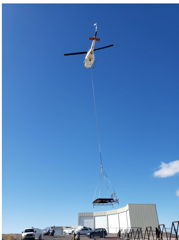
Figure 8.1.: Deployment of a scintillator on November 15, 2022. For environmental protection, the scintillators are flown to the deployment site with a helicopter [67].
