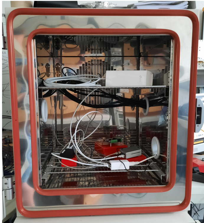
Figure 5.9.: New network components in temperature chamber. On the upper grate the WLAN antenna, on the lower grate on the left the black Ethernet switch, on the right the Raspberry Pi in its gray case, in the back the smart relay card is visible.
