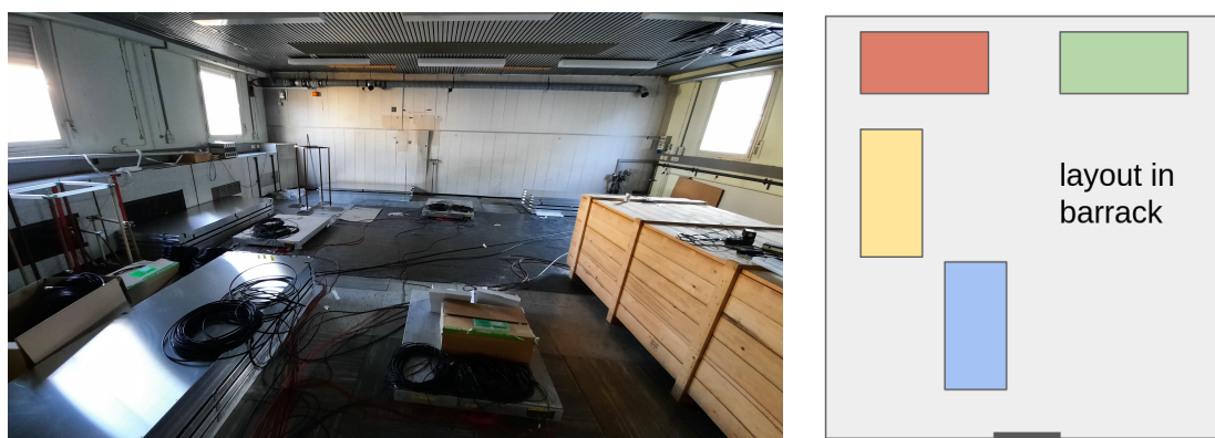
Figure 5.1.: Position of the panels in the barrack. Left: Picture of the barrack with the scintillators during the measurements at KIT. The wooden box on the right is used to heat up the scintillators (section 6.2). Right: Sketch of the positioning of the panels inside of the barrack. The blue rectangle corresponds to the scintillator stack visible at the bottom left.
