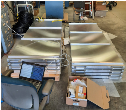
Figure 7.4.: Two scintillator stacks at the CRC. Left: Picture of the setup with two piles. Center and right: Sketch to show the order of the scintillators in the one and two pile setup. During the two pile setup, the spare panel #186 is put to the side to have the same amount of shielding from the top.
