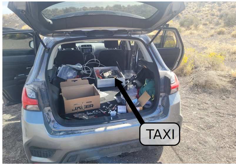
Figure 7.11.: TAXI set up in the car in the field. TAXI was powered via the car battery. Behind TAXI, the white Ethernet cables to connect the Raspberry Pi and a laptop are visible. The trunk of the rental car was repurposed into a workbench. Picture from [86].
