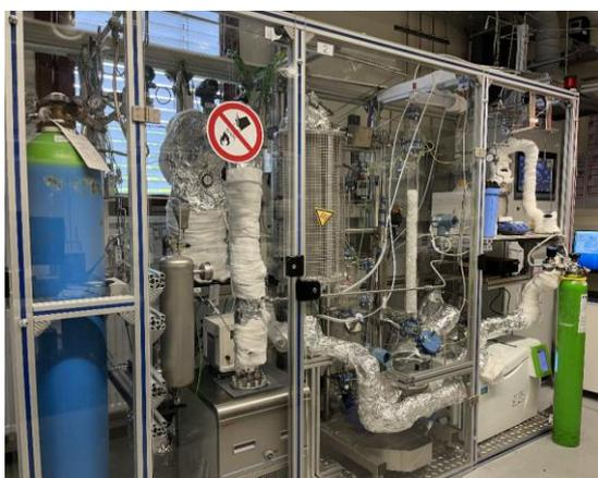
Figure 10: MEDENA mini-plant for the dehydrogenation of methanol to anhydrous formaldehyde at KALLA (Photo: M. Kamienowska)
