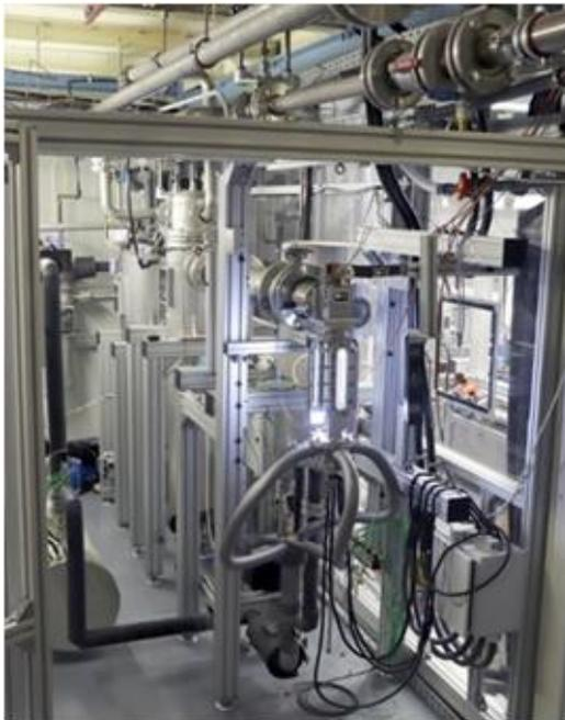
Figure 1: Critical-heat-flux On Smooth and Modified Surfaces – Low pressure loop (Test Facility COSMOS-L)
