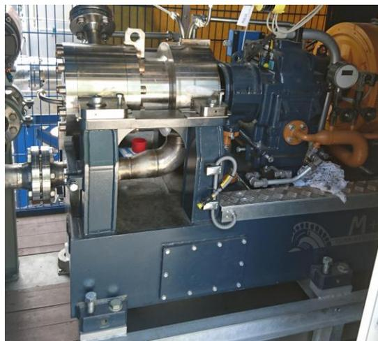
Fig. 4: Turbine with gearbox and generator
