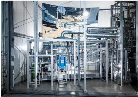
Figure 12: Demonstration plant built at KALLA: detailed picture of the methane pyrolysis set-up.
