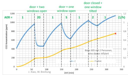
Figure 4. Analysis of venting strategy and infection probability using the point model
