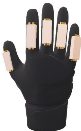
Figure S2-16. Schematic of fabric glove (black) with five strain sensors (pink).
