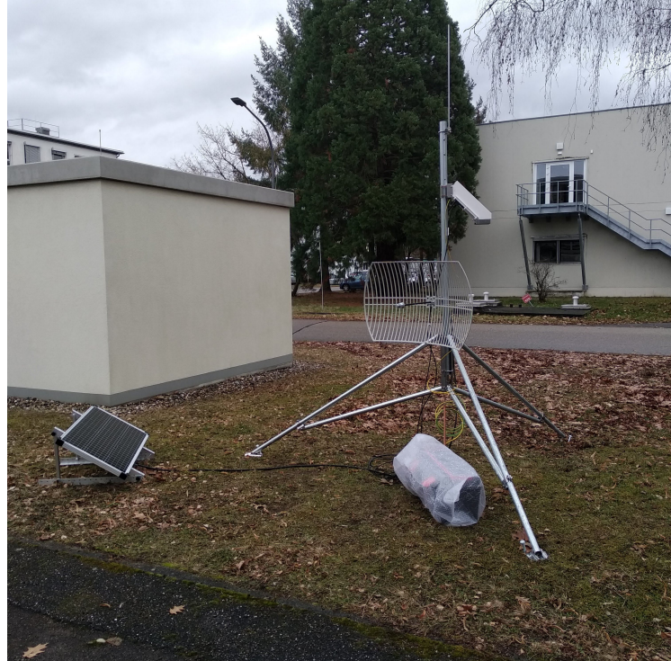
Figure 2. The test setup of the new EFM stations at Karlsruhe Institute of Technology. The tripod holds the EFM at the top and the WiFi antenna below. On the ground the electronics box and the solar panel are placed.
