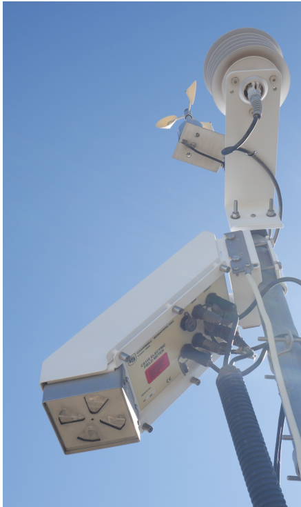
Figure 1. The EFM and other weather sensors at AERAWs. The rotating vane shielding the sensor plate is visible.
