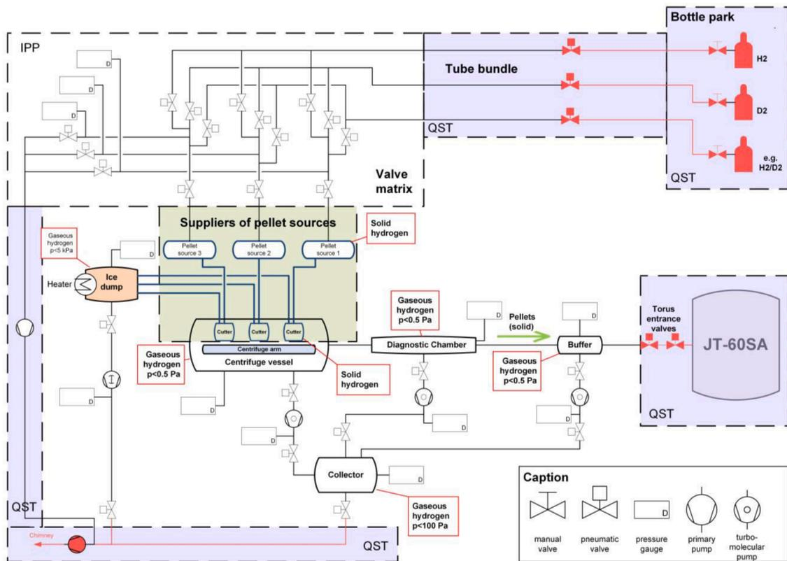
Fig. 3. Block diagram of PLS in testbed at IPP Garching. The system is displayed with the three maximum possible pellet sources (initial delivery will be only two of them). The boxes labelled with “QST” are expected to be provided at Naka site under responsibility of QST. The components in the box “Suppliers of pellet sources” are to be provided by PELIN. The Valve Matrix is an IPP contribution, the remaining parts: centrifuge and vacuum system is up to SENNER.
