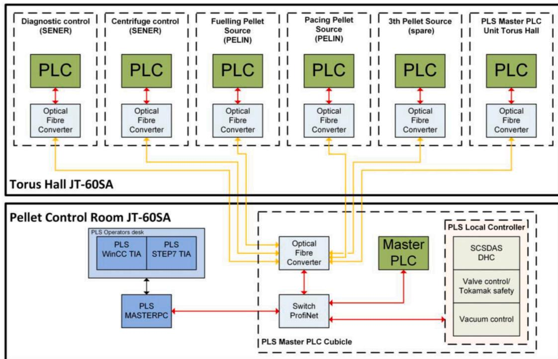
**Fig. 1.** PLC architecture block diagram. The devices are connected via PROFINET using optical fibres (yellow) in order to provide electrical potential separation. The operators' desk is located in the pellet control room as well as the CPU of the MasterPLC. The interface to JT-60SA control systems DHC (density and heating controller) and SCSDAS (supervisory control system and data acquisition system) provided by the PLS local controller, serving as interface.
