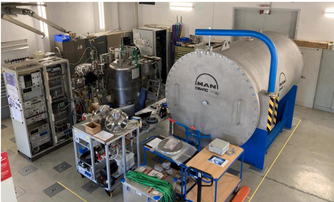
Fig. 4. IPP pellet lab with 10 m<sup>3</sup> vacuum tank ready to host PLS for JT-60SA. Primary vacuum setup is installed on basement.
