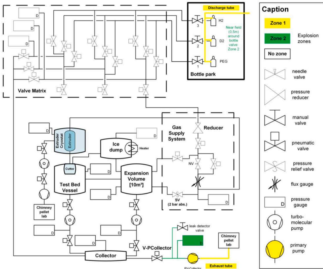
**Fig. 2.** Block diagram of test bed configuration to host one single pellet source. One channel of the Valve Matrix is used to provide gas to the pellet source gas supply system. The pellet source is mounted on the test bed vessel. Green elements are stated to be zone 2, yellow ones being zone 1.
