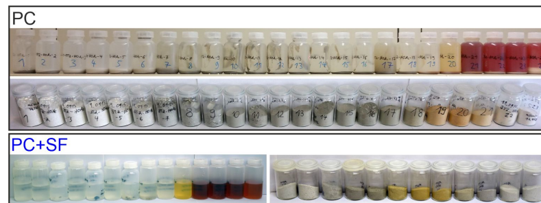
Figure 1. Photographs of selected suspensions before filtration and of the solids after filtration for PC, as well as some of the liquid and solid fractions after filtration for PC + SF (for each series with decreasing pH from left to right).
