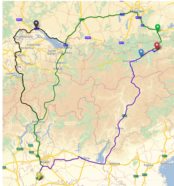
Figure 11.4: Optimal paths of an example query from northwestern Austria to northern Italy, slightly south of Milano. The source is indicated by a red, the destination by a yellow marker. The other markers indicate the parking locations along the respective routes. The blue route in the east has the shortest driving time, around 10.5 hours, but the latest arrival. It schedules a waiting time of seven hours during the night driving ban at a parking location of rating 4 and afterwards takes the fastest route to the destination. The green route in the middle arrives an hour earlier at the destination but the driving time is over two hours longer. This route includes three hours of waiting at a parking location of rating 5. The black route in the west takes 16 hours to drive, includes only a few minutes of waiting and arrives six minutes before the green one.
